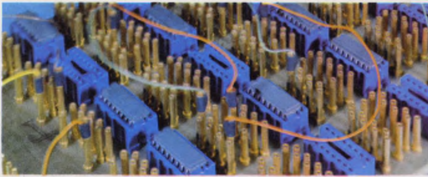
For breadboarding small quantities of ICs, this panel from Augat is handy, because interconnections are made with standard wire jumpers.
