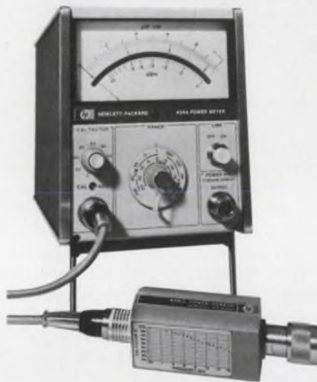
The 435A power meter's internal RF power reference provides added confidence in overall measurement accuracy.
