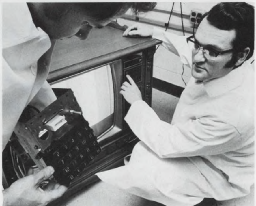
ICs and discrete solid-state components are taking over in color television sets like this GTE Sylvania receiver. Here, engineers check the varactor tuning.
