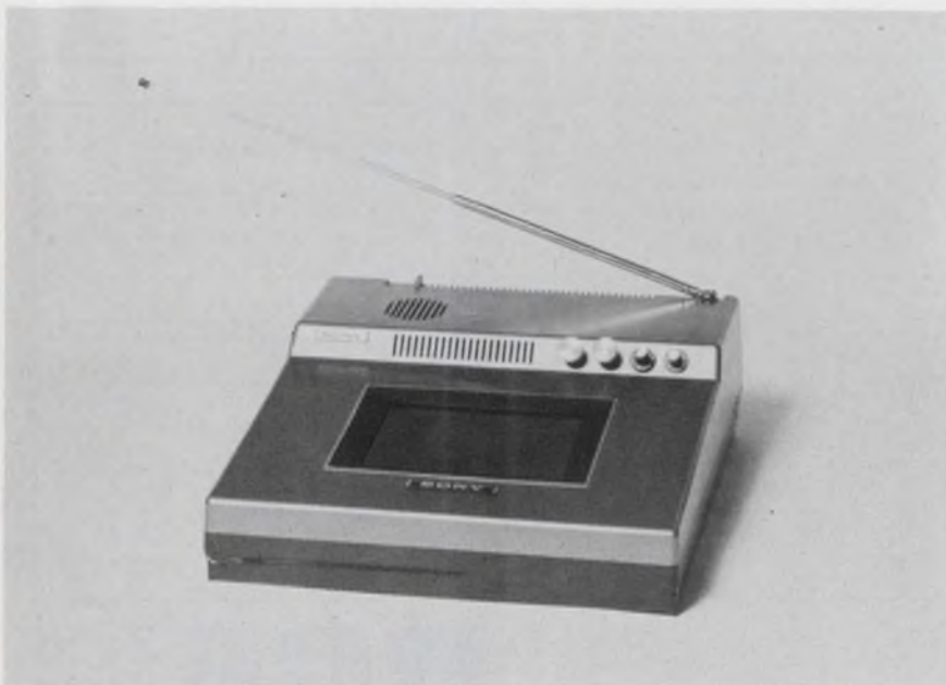
Prototype dc plasma-panel TV from Sony consumes 90 W of power—10 W for the panel and drivers and 80 W for the rest of the electronics.
