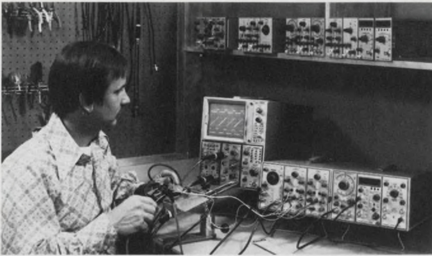
A leading example of synergistic instrumentation is the Tektronix TM 500—a modular system of counters, DVMs, signal sources and other instruments that share a common enclosure, power supply and other circuit elements.
