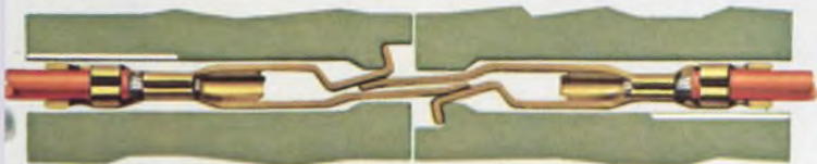
Positive wiping action and gold-over-nickel plating of miniature DUALATCH contact ensure excellent electrical and mechanical performance.
