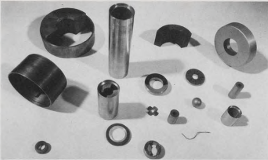
Rare-earth magnets , originally designed for use in microwave tubes, are now being used in motors, generators, watches and meters.
