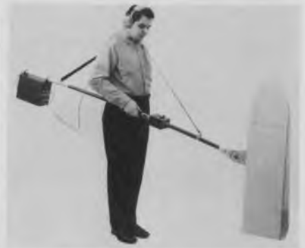
High-resolution radar developed by Calspan weighs less than 20 pounds and sees below the ground up to two feet.
