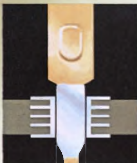
Solder band is pulled into through-hole with just enough force to retain it during reflow.
