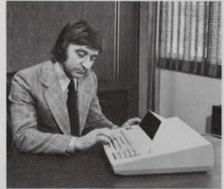
The MCM/70 desk-top computer is the first portable one capable of using the powerful APL language.
