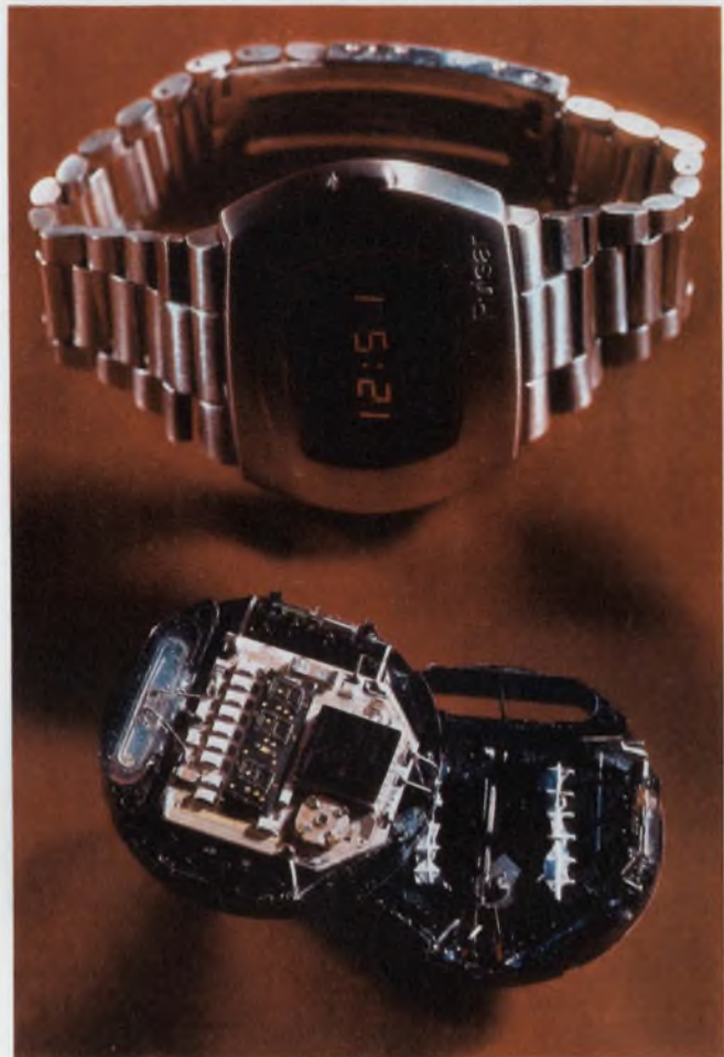
A clear Dow Corning silicone gives this Pulsar watch crystal protection against shock, while black silicone mounts the LED display. The black silicone protects the display against shock and also gives higher contrast.
