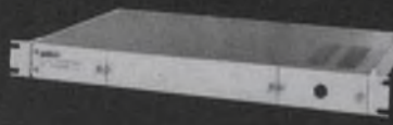
MODEL 610 COUNTDOWN UNIT Used for locking sync generators to a local color subcarrier signal, and framing rasters generated by different sync generators. This unit generates a 31 468 kHz signal from a 3 579545 MHz source.
