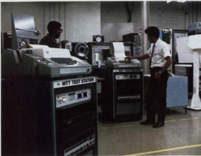
Computer-based test system built by General Automation checks magnetic tape transports for quality, accuracy and reliability. It also checks mechanical functions, such as response time, accuracy of speed and reliability.
