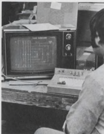
TV set serves as a CRT for Quindar's supervisory-control system. It can display all or portions of an electric utility network.
