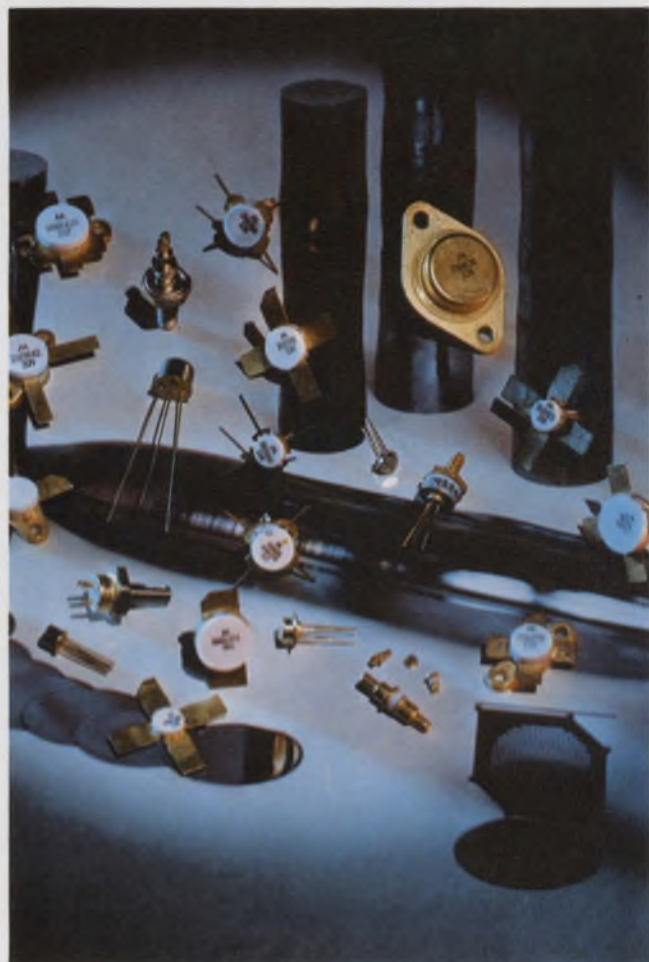
Motorola offers rf transistors in a variety of packages, including TO-3 types and its SOE configuration.
