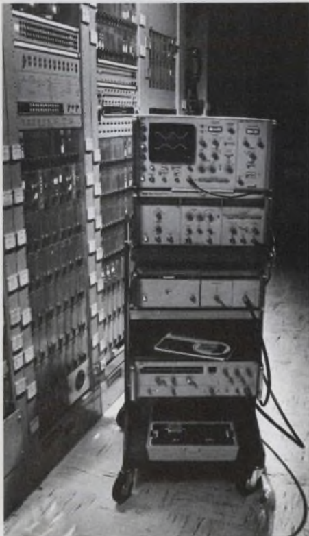
HP's microwave link analyzer is ideal for optimizing radio relay link performance.
