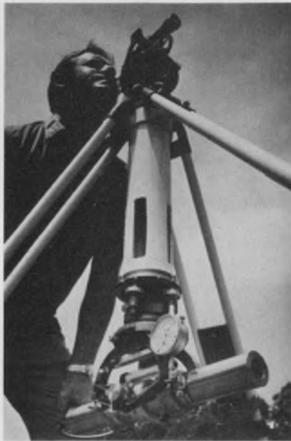
Helium-neon construction lasers, like this Metrologic system, are becoming more versatile.
