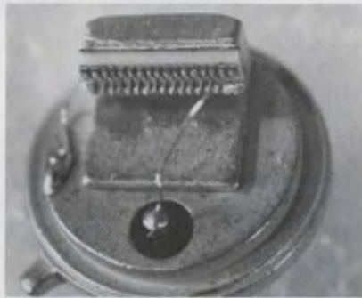
RCA's 15-diode linear array provides a peak power output of 75 W.
