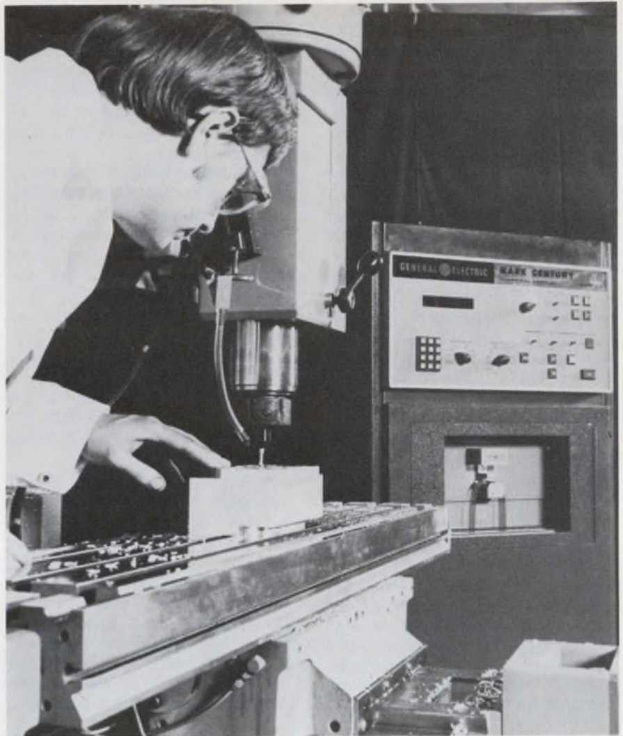
General Electric's new Mark Century 550 Series numerical control is offered in two versions: 2 or 3-axis controls for contouring and positioning applications and 2-axis contouring controls for turning machines.
