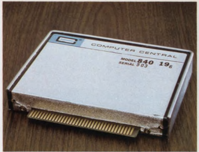
A differential d/a, the Model 840, made by Computer Central. It gives an analog-signal output that is proportional to the difference between two parallel BCD inputs.
