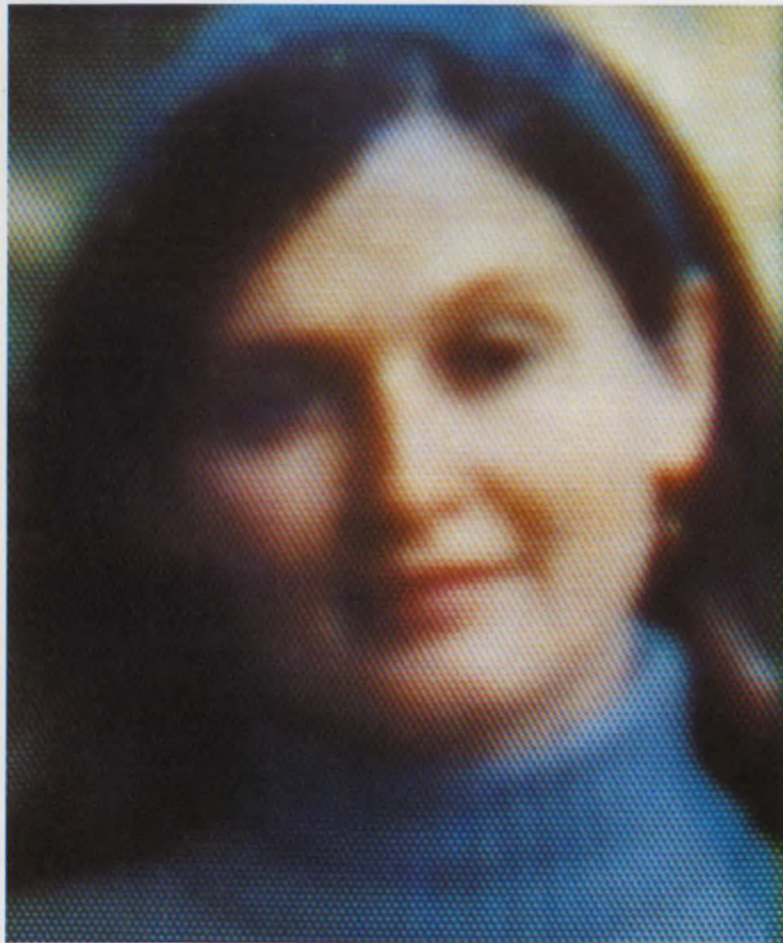
Color image formed by Bell Labs' CCD television camera reveals that the principle is sound but the resolution is poor. Higher-resolution cameras are expected to be available before the end of the year.
