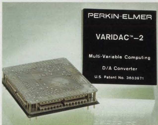
A two-channel d/a made by Perkin-Elmer, the only company to produce a multiplying d/a that uses an auto-transformer rather than a resistive ladder network.
