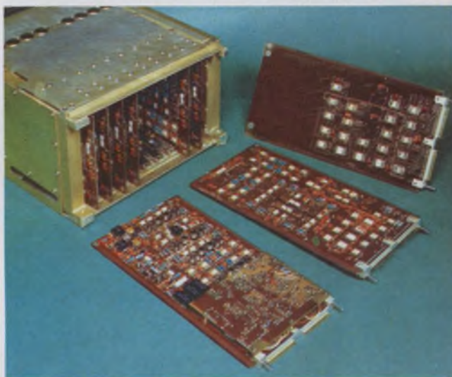
Singer-Kearfott's SKC-2950 is an eight-bit militarized a/d converter. It features a 25-ns conversion time and has two channels.
