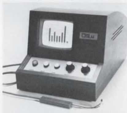
Probes of a Computer Synektics Micro-Sum monitor connect to the circuits of system being measured. CRT shows computer element activity.
