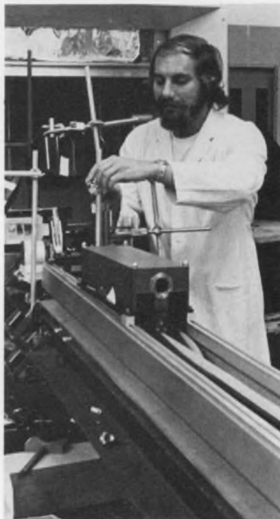
Using a high power infrared laser and a copper sulphate sandwich as a target, Kepros is said to have produced the first X-ray laser.
