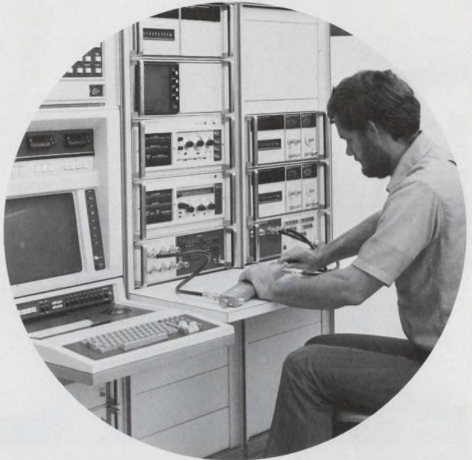
Shown here testing a UHF component, the HP 8580B serves as a cost-effective production test station.
