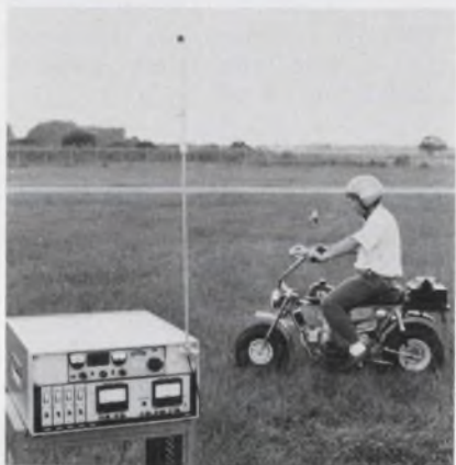
EMR telemetering system on board the minibike transmits field test data to the portable station at left.
