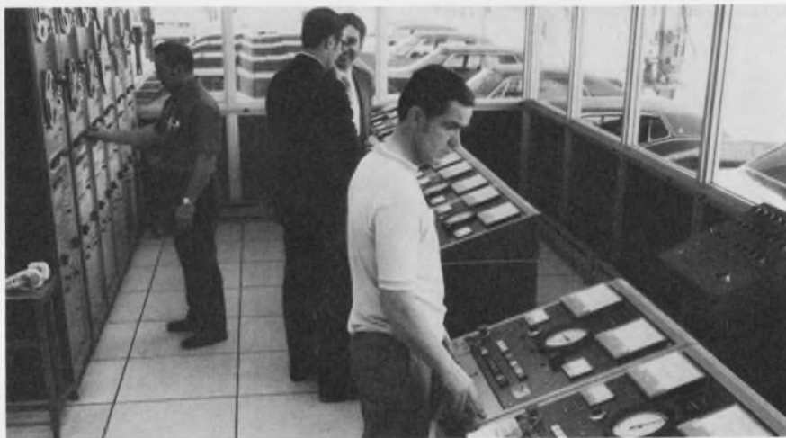
Multiple test stands at Ford's Allen Park facilities use computers and magnetic tape storage to acquire and process test results. Each of the test stalls is operated and monitored from its own control console.
