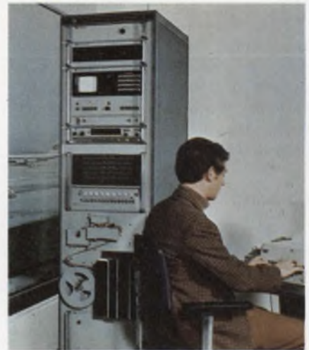
Hewlett-Packard airport monitor checks jet noise levels fast enough to warn pilots of excessive levels.
