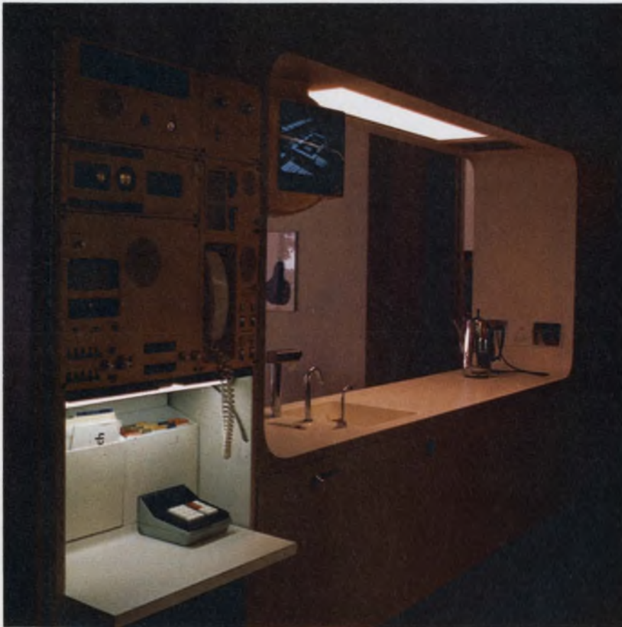
Prototype of a futuristic kitchen designed by Westinghouse Electric Co. contains a communications command post which incorporates automatic telephone dialing, a tape recorder, AM/FM radio, closed-circuit television and controls for temperature, humidity and a home security system. A cable TV hookup is also under consideration.
