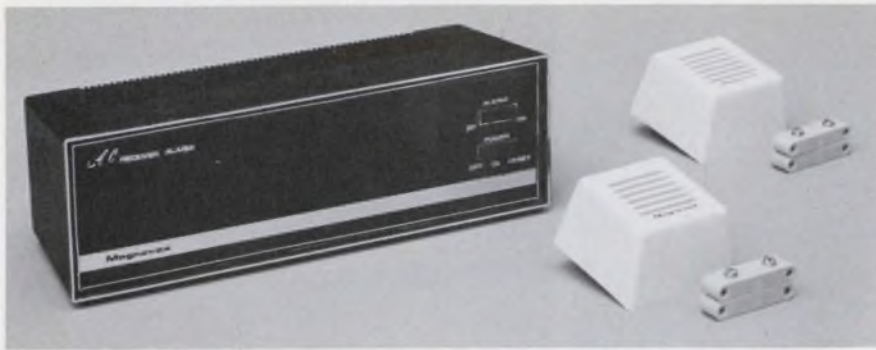
Carrier-current alarm by Magnavox uses ac house wiring to connect sensors with an alarm latching circuit.
