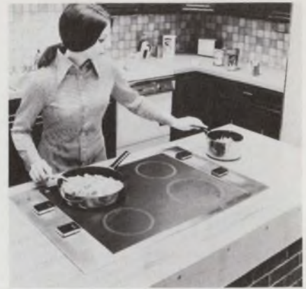
An induction range whose top always stays cool to the touch is being sold by Westinghouse. Coils of wire, under the black ceramic top carry a 25 KHz ac current. When an iron or steel pot is placed over a coil, the pot couples with an oscillating magnetic field created by the coil and the pot heats up.
