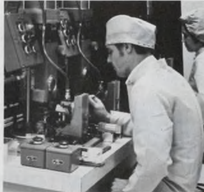
P&B precision assembly machines make it possible to control gap variance in reeds to within 2/10,000ths of an inch. (1/10th the thickness of a human hair.)
