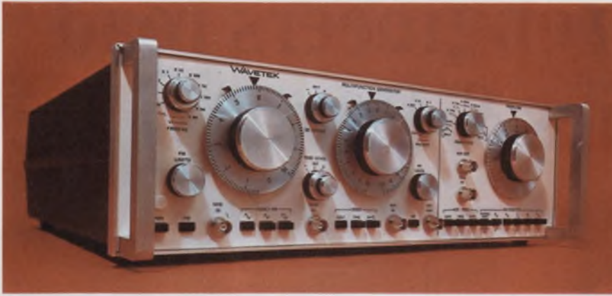
Dial calipers show the manually set limits for FM and AM in the $1495 Wavetek 146, which includes a separate section for generating modulation waveforms.
