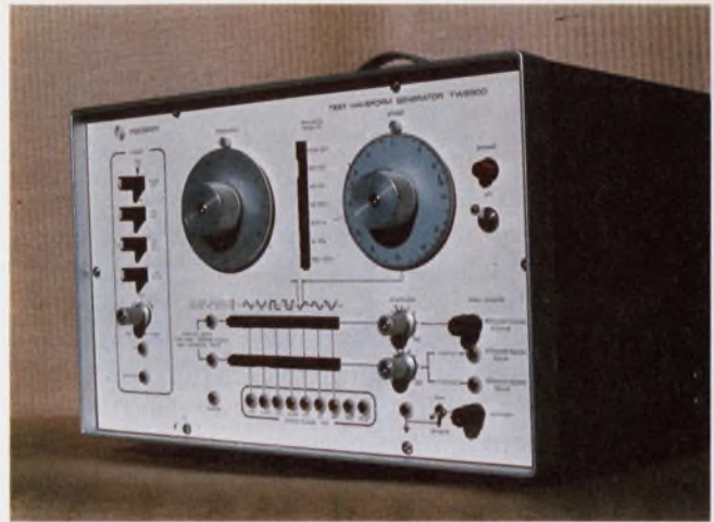
Five sine waves, displaced from a reference by 0°, 90°, 180°, 270° or, continuously variable from -180° to +180°, are available in Feedback's TWG-500. The $1650 instrument—for 10 mHz to 100 kHz—also has quadrature square waves and triangles.
