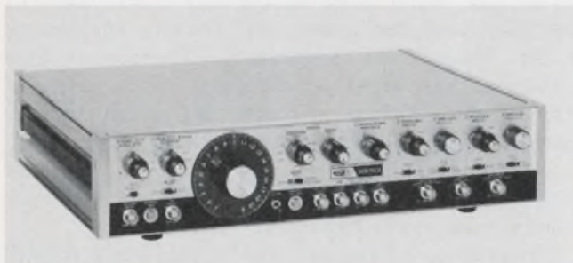
Independent waveforms are available at two separate outputs of the Datapulse 410, a $995 generator with a sweep range of 1000 to 1 over 200 \mu Hz to 2 MHz.
