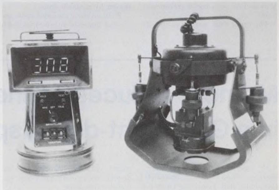
New digital Hall-effect sensor is being used in this marine compass system. The compass assembly, at right, is hydraulically damped. The binnacle display and control unit, at left, is about 12 inches high.
