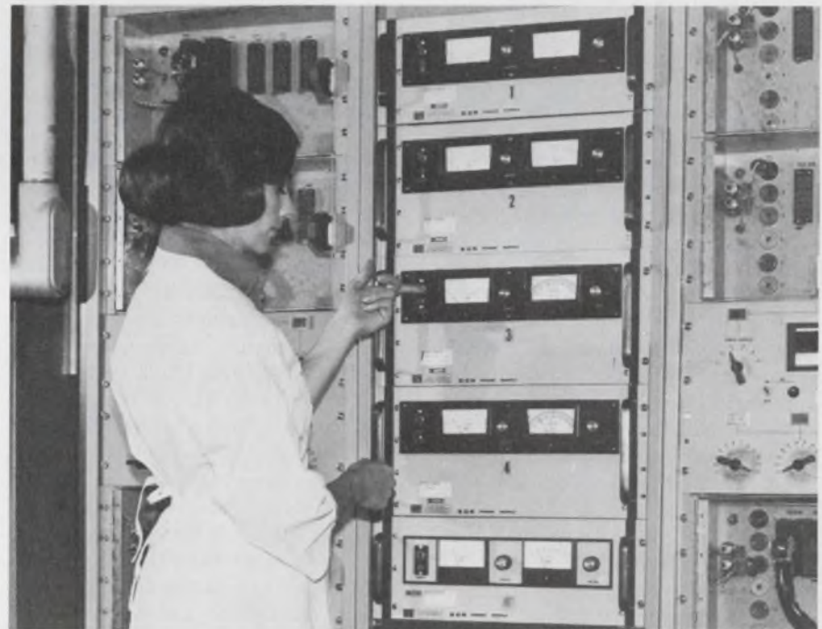
Five of E/M's 5 KW SCR Power Supplies are used in General Electric's electrolytic capacitor aging system.
