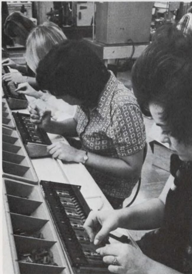
Module assembly carriers minimize handling and speed material flow in "high speed assembly/solder line."
