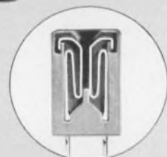
Cross Section Shows How a Continental Contact Hooks on Top of Connector Molding for Permanent Grip.
