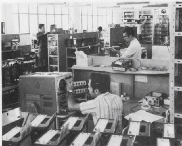
A line of frequency counters undergo inspection and "burn-in" at Monsel's final test department.
