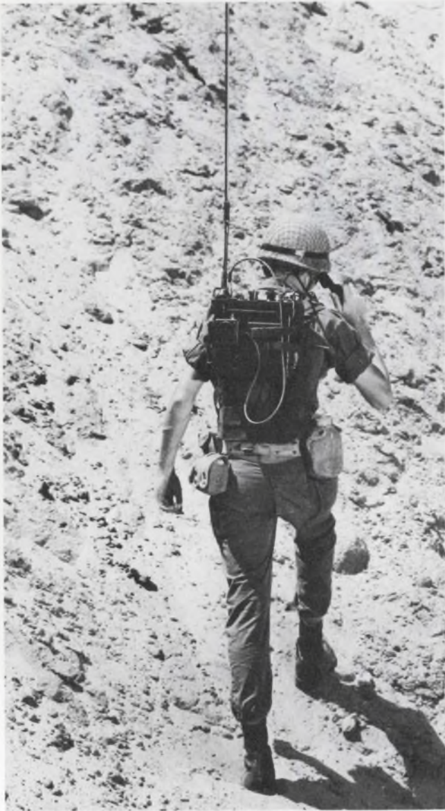
Israeli soldier carries an AN/PRC-77 back-pack radio manufactured by Tadiran Israel Electronics Industries Ltd. The unit includes a loudspeaker-assembly that enables a commander to listen in on the conversation.
