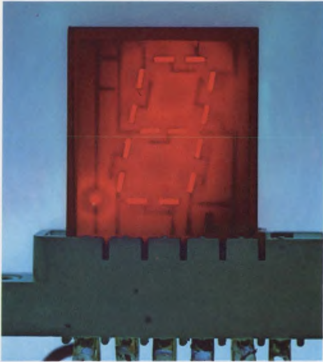
The first large LED readout, this Litronix device with 610-mil characters, plugs into a conventional PC edge connector making special sockets unnecessary.
