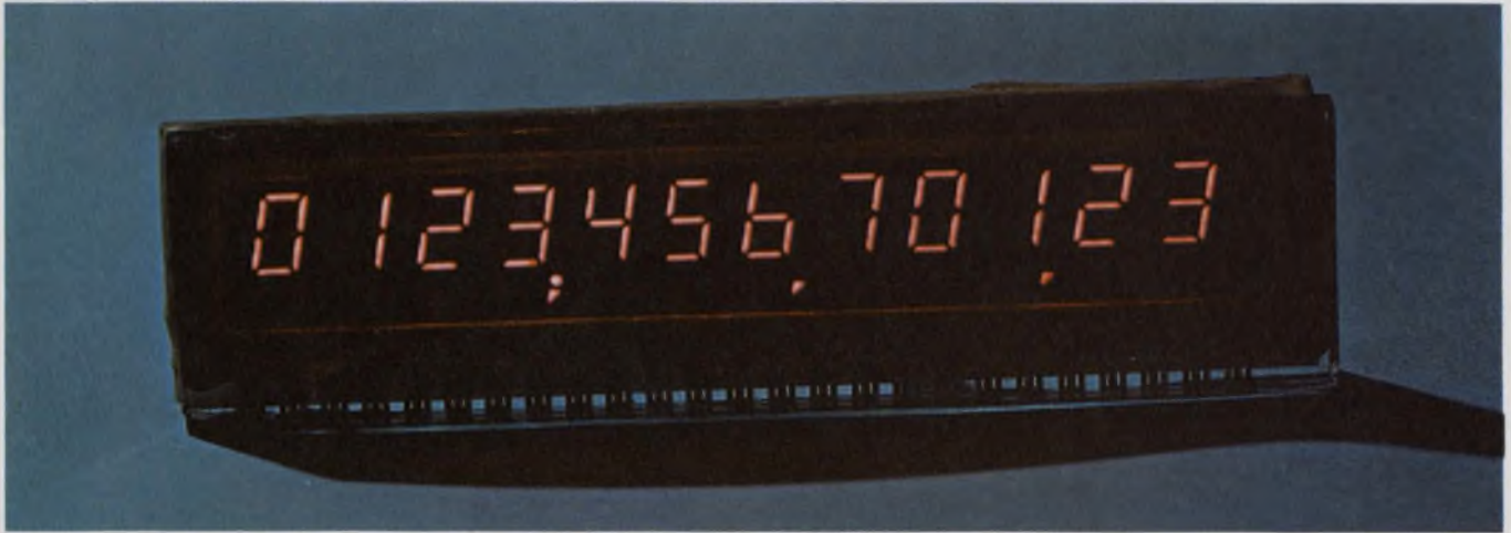
Gas-discharge numerics in Burroughs' Panaplex II are formed of bars, printed all at once, on a single substrate.
