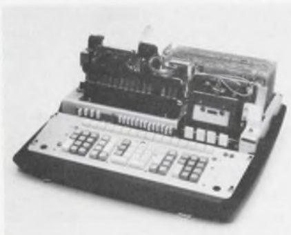
This microprogrammed Model 500 Wang calculator (left) has an 88-k bit braided-wire control ROM (right) that shrinks the machine to desk size.
