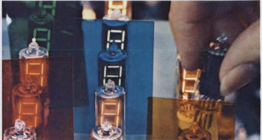
Directly viewed filaments in RCA's Numitron are operated at much lower temperatures than conventional lamps, so they can last a long time. With suitable filters, they can show a wide range of color.
