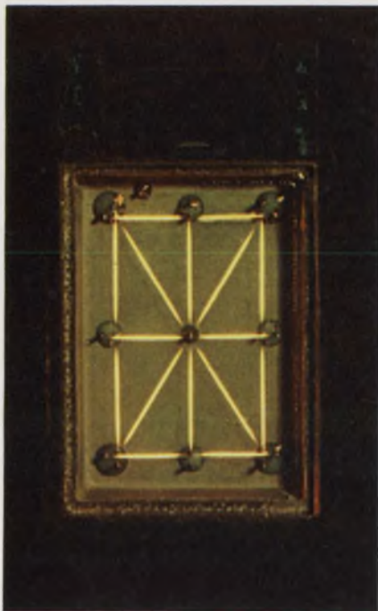
Double-post construction at the corners of this 16-filament, full-alphanumeric readout from Pinlites eliminates corner gaps.
