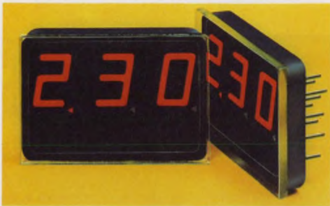
Small gas-discharge planes with three, two or 1-1/2 digits consume very little power. They're from Sperry
