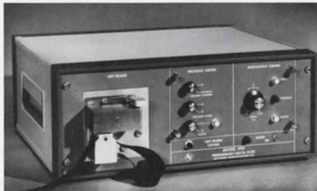
the Electronic Communications' filter (right) offer fully programmable filter characteristics. A set of numbers, which can be changed easily, completely determines the desired filter function.
