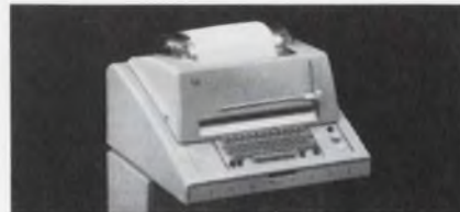
model 35 series: A rugged, heavy-duty line of 100 wpm terminals. Uses ASCII.
