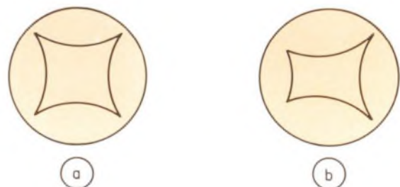
1. A square trace is distorted by a single gun CRT into the pin-cushion of "a." An off-axis gun, as found in a multigun tube, causes additional keystone distortion (b).
