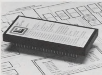
Standard MOS/LSI devices, such as this data communicator developed by Larse Corp., may eventually replace pneumatic equipment now used for control functions in factories.
