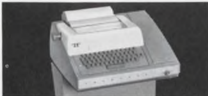
model 33 series: An extremely low-cost 100 wpm terminal line. Uses ASCII. The most widely used terminal in time-sharing systems today.
