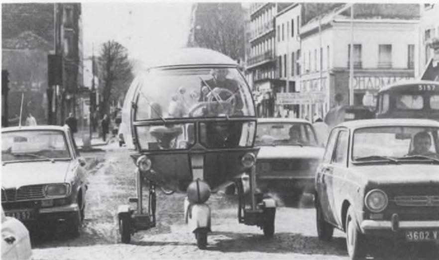
"Car of the year 2000," which Honeywell of France used to demonstrate its line of microswitches. Pushbutton-devices maneuver the vehicle.
