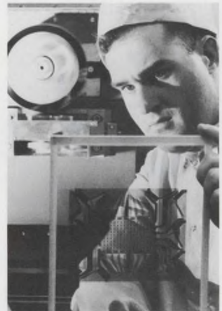
Laser beam and 10-sided rotating mirror cut time to one-sixtieth for drawing mask patterns for ICs.
