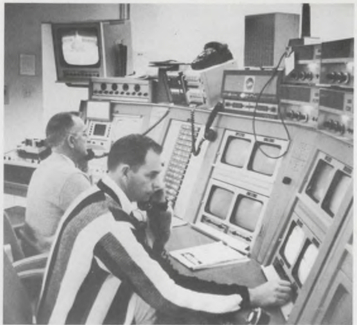
Flight Vision Room console allows test engineers to watch flights from a number of vantage points on a number of TV screens. The 80-inch lens shows planes 150 miles out.
