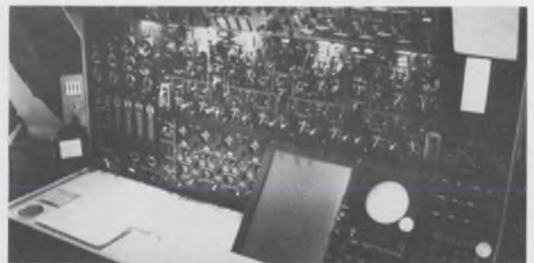
Flight crew compartment seats six—two pilots, navigator, engineer, and two observers. Upcoming tests will concentrate on the instrument landing system, radar altimeter, inertial navigator and engine readings. The display for the plane's automatic test system is at the lower right of the engineer's console (above).
