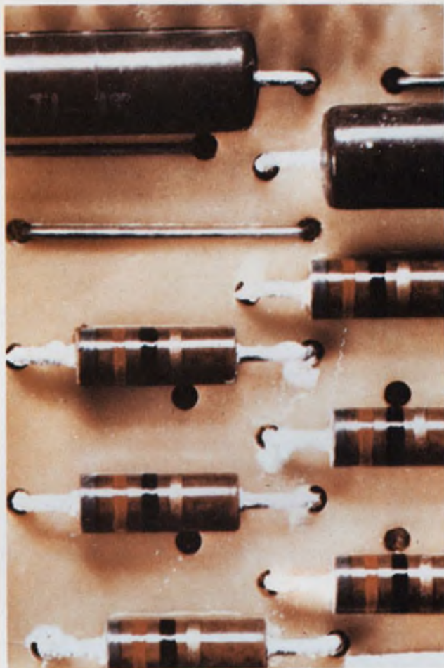
Cleaning in trichloroethylene only was the procedure used with this PC board. Since the procedure left all ionizable materials behind, all lead-rich surfaces were attacked by chlorides. The white corrosion products that formed can be seen on the leads. Close observation indicates leakage paths across the board surface under high humidity conditions.
