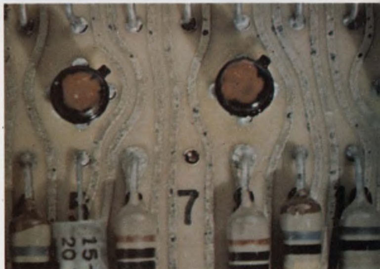
This printed-circuit board appeared clean after manufacturing. However, corrosion spots developed with time. They proved to be etching and plating solution residues that bled to the surface.
