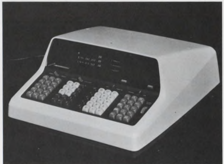
Multi-function desktop calculator , which offers sub-routine capability, stores 392 program steps, p. 130.
