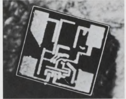
On-chip Hall generator digitizes its dual 10-mA output, p. 138.
