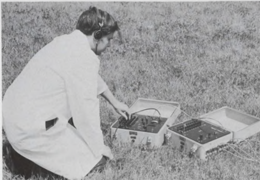
A 10-channel alarm system built by DEI Industries warns of intruders within a 3.6-million-square-foot area. Called AIDS-10, the system employs buried geophone sensors that are linked by wire to a multiplexer.
