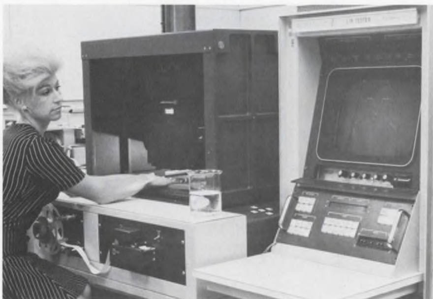
IR temperature-sensing instrument , developed at Autonetics to detect flaws in microcircuits, detects minute temperature differences on the surface of the human body and displays them on a CRT screen.
