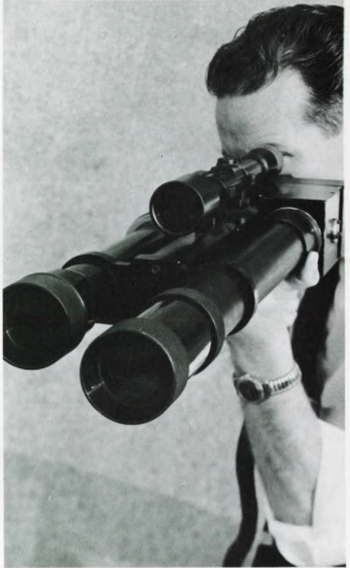
Counting backward eliminates undesired early returns in laser ranging measurements. Here an engineer sights a Colidar Mark II range-finder. p. 78
