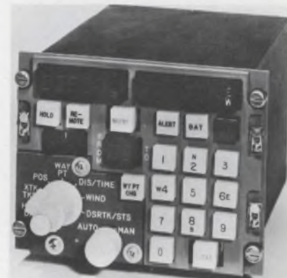
Carousel IV inertial navigation system, built by AC Electronics, is off only two miles on a 4000-mile flight, Pan Am says. The two units (a third is on hand as a spare) tell the pilot his position, distance to destination, wind velocity and direction, drift angle and ground speed.
