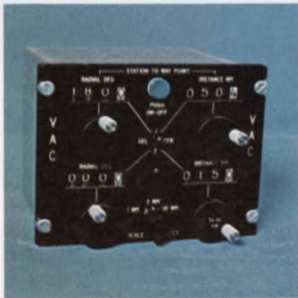
A more complex control panel and rectilinear indicator is featured in Butler National's Vector Analog Computer for the company's area-navigation system.
