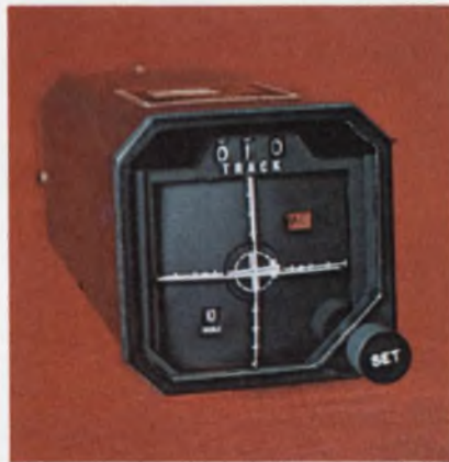
A more complex control panel and rectilinear indicator is featured in Butler National's Vector Analog Computer for the company's area-navigation system.
