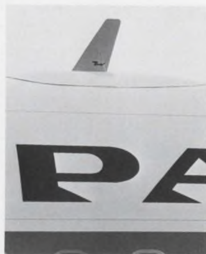
Blade antennas for the conventional vhf transceiver emerge from the top of the fuselage or from the belly.
