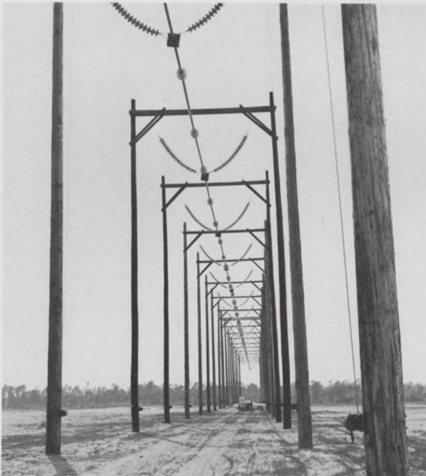
Long-wire, electromagnetic pulse (EMP) test facility of Martin Marietta at Orlando, Florida. The "wire" is a 1000-foot dipole antenna with a spark gap in the center. Used to determine effect of nuclear EMP on military electronics equipment, a 20,000-ampere discharge produces a giant pulse.
