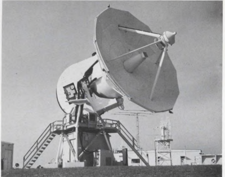
This 30-foot diameter antenna is part of NASA's Unified S-band communications system. It is used for near-earth operation—tracking and communicating with the Apollo spacecraft during launch.
