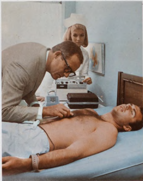
Analog data communication: Electrocardiograms can be transmitted over standard telephone lines with a special Bell Dataphone set.
