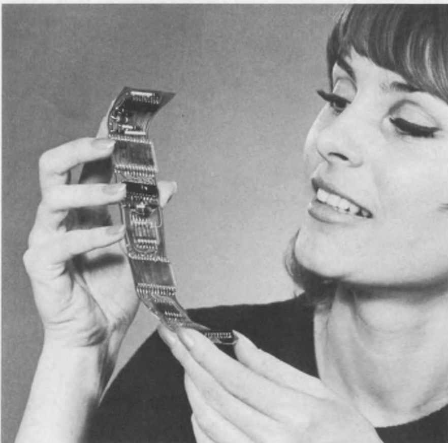
Handset portion of an experimental all-electronic "telephone of the future," designed by Northern Electric Ltd. of Canada, houses integrated circuits and thin-film components.
