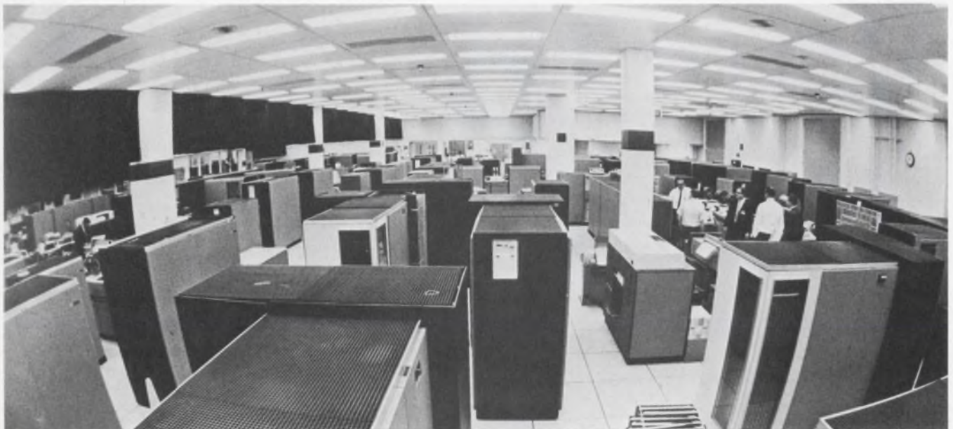
RTCC, the Real Time Computer Complex, at NASA's Apollo Mission Control Center in Houston is one of the world's largest digital processing facilities. A portion of the five IBM System/360-75s employed is shown in this
