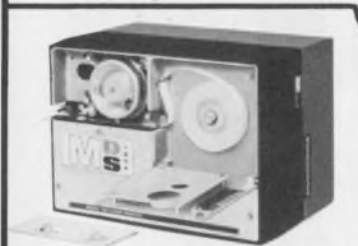
With cover panels removed, miniaturization of the 120A is easily seen.
