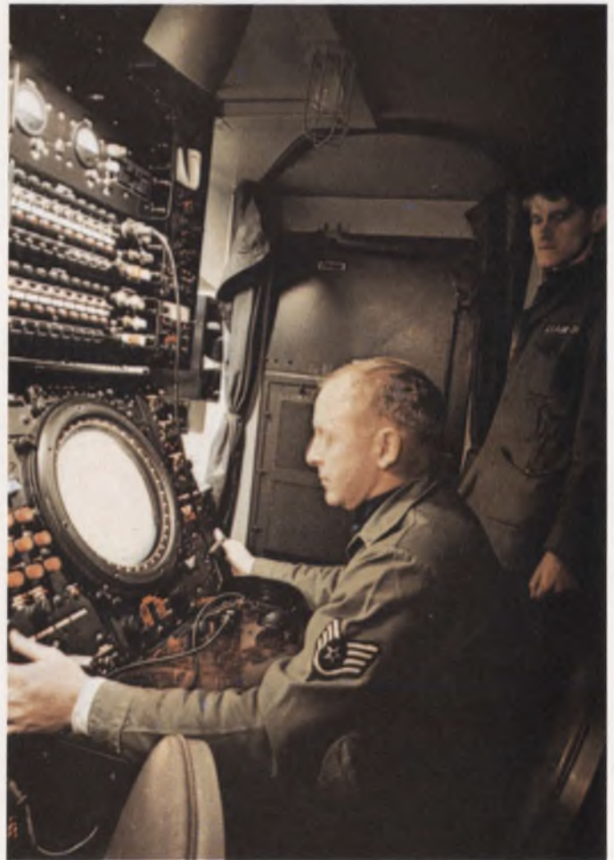
Radar operations van, AN/TSQ-61, for the Air Force AN/TPS-44 search radar, includes five videos, remote controls.
