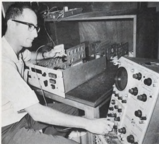
6. The author, Israel Urieli, is testing the 1-MHz comparator diagrammed in Fig. 5.
