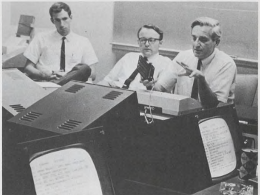
SRI researchers demonstrate the use of interactive computing with graphics for group discussion of a system design. General files, as well as individual files, all in the process of development, can be examined, modified or added to by the group. The system being designed is the system they are using.
