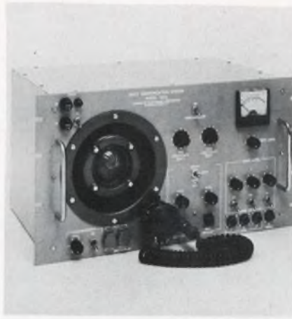
Helium speech unscrambler to eliminate Donald Duck talk operates in real time, is completely solid state, provides frequency shifting in two channels, 0 to 1000 Hz. Device is made by Integrated Electronics.
