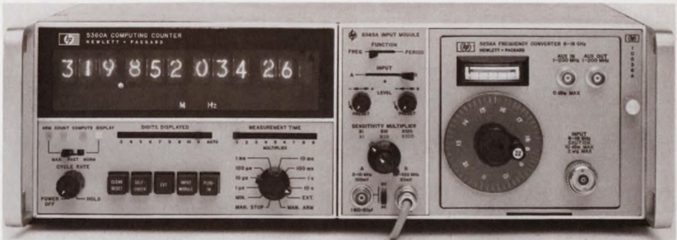
Multi-function 320-MHz computing counter processes measurements like desk calcula-
