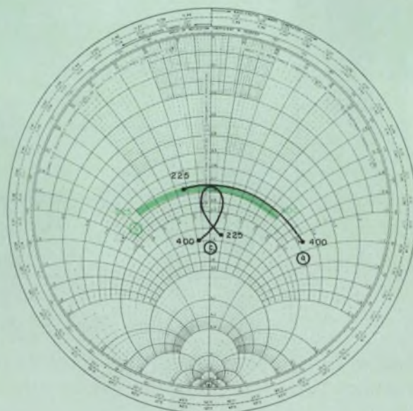
2. The large-signal input impedance of an ITT 3TE445 transistor is shown by curve (a) from 225 to 400 MHz. In (b), the effect of putting a capacitor in series with the base is shown. Curve (c) results when a shunt pole (Fig. 3) is added. All curves are normalized to a 1-ohm line.
