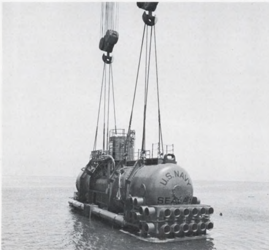
Sealab III's helium gas breathing-mixture is vital for the aquanauts but gives electronic components the bends.
