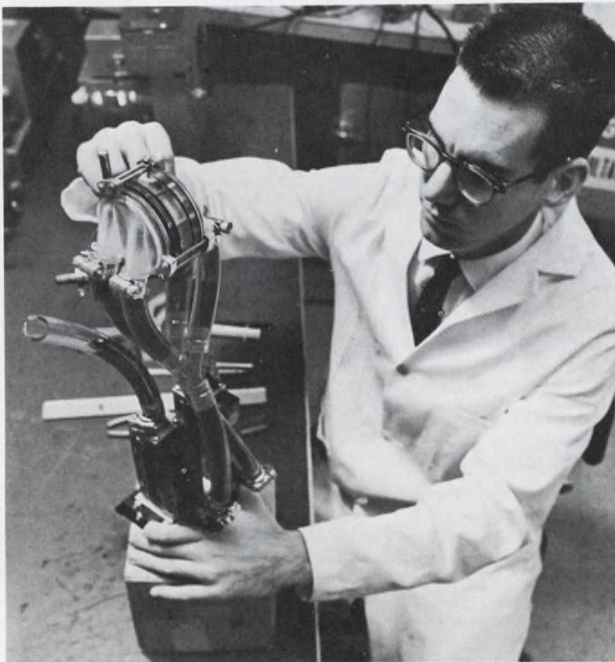
An early version of a piezoelectric heart pump made by Hamilton Standard's Biomedical Division. Pump is at top, ventricle at bottom.
