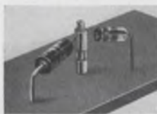
Solder one end to P/C board and attach lead to other end.
