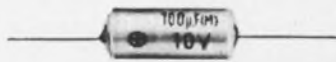
Type TSX encapsulated in metallic case and sealed with epoxy resin Standard voltage rating: 3V, 6V, 10V, 15V, 20V, 25V, 35V D.C. Standard capacitance value: 1 MFD to 220 MFD (E-6 series)
