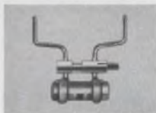
Solder ends to terminals of another component.
