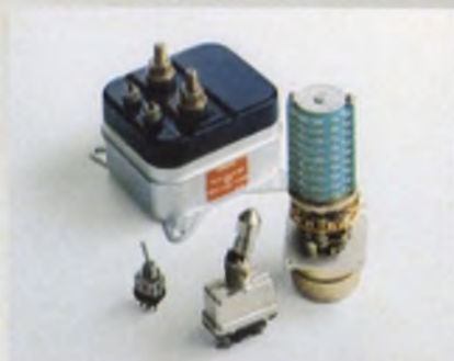
Some of our relays and switches for ground, sea and airborne installations around the world: Miniature and standard-size, positive-action toggle switches built to the requirements of MIL-S-8834, Shallcross rotary switches (to MIL-S-3786). Hermetically sealed power relays and 175-amp generator contactor (to MIL-R-6106).
