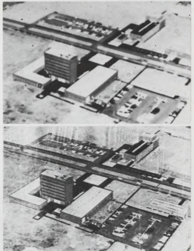
1. Atmospheric turbulence blurred this aerial scene (top) but spatial filtering with an inverse Gaussian filter cleaned up much of the distortion (bottom). Note particularly the improvement in fine detail, such as the windows.
