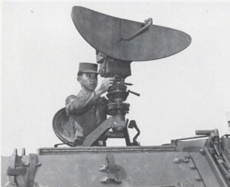
The Vietnam conflict has shown the need for improved types of small tactical radars for detecting personnel movement and for enemy mortar and artillery location. Shown is the AN/PPS-5 built by Airborne Instruments Laboratory.
