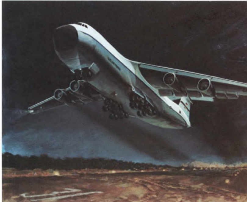
Artist's conception of C-5A in flight. Aircraft is designed to carry 100,000 pounds of payload for 6300 miles, and up to 265,000 pounds for shorter distances. It will be 82 yards long with a wingspan of 74 yards.
