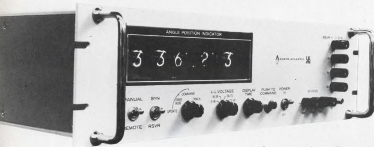
Resolver/synchro-to-digital converter tracks to 2000°/s. The six digit instrument has an updating time of 125 ms (for a 180° input step). In addition, the unit has a Velocity Constant of 20,000 to 1, a variable 0.3 to 3 second display time and three operating modes. Page U134.
