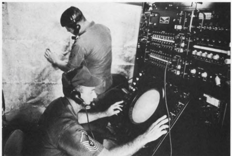
The radar operator inside the AN/TSQ-61 van spots approaching aircraft on the AN/TPS-44 search radar's remote indicator and passes position data on to an assistant, who plots the coordinates.
