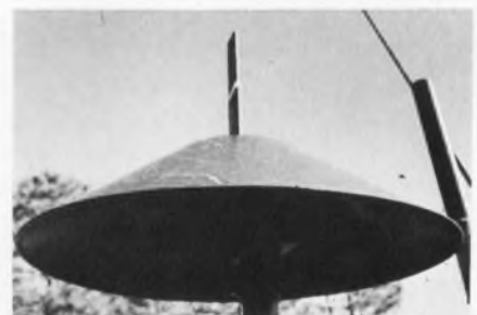
"Coolie hat," fabricated at Eglin Air Force Base, Fla., solved a poor uhf antenna pattern caused by an irregular ground plane. The irregularity was created by the hood of the jeep on which this AN/MRC-107 is mounted.
