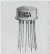
RCA CA3035 wide-band high-gain ampl. in TO-5 package. Price $1.50 (1,000+)
