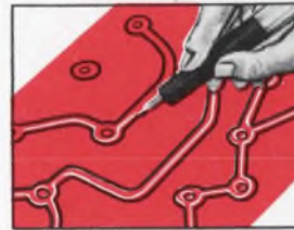
With sharp blade, outline the areas to be masked. Do not cut through the backing sheet. The Ulano Swivel Knife does the job quickly, easily.
