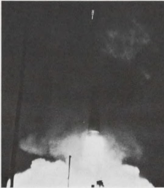
A Sprint roars skyward in a test, scattering bits of debris from its silo cover. It was popped from its silo by a propellant gas before its first stage ignited. Acceleration of the 27-foot long missile is over 100 G's.
