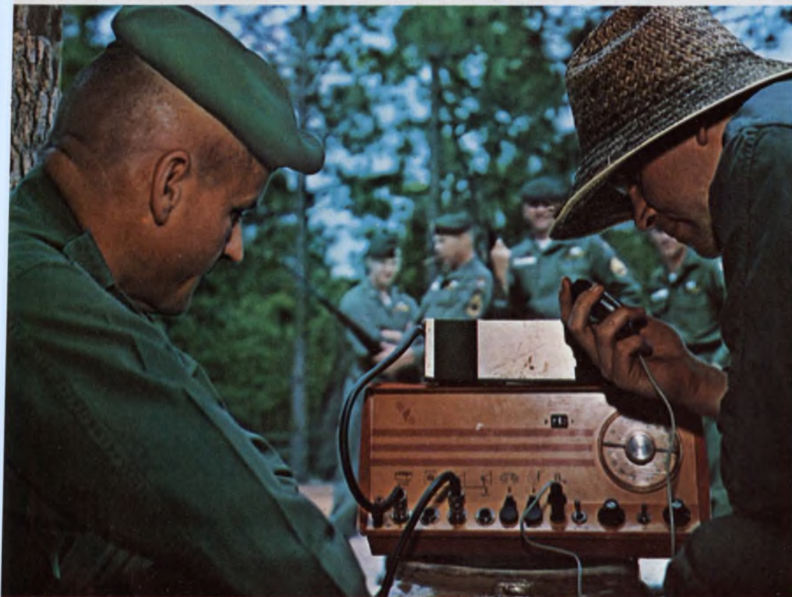
A hamlet communications system is provided by this versatile Arvin Industries equipment. The use of the set (Model 63CRA11) as a public-address system, to allow a hamlet chief to address the villagers, is demonstrated here. A battery box is shown on top. As a radio, the set covers 535 to 1605 kHz. It also works with a tape recorder or phonograph. Note that all sockets are marked by sketches, so that natives can learn to operate the set.
