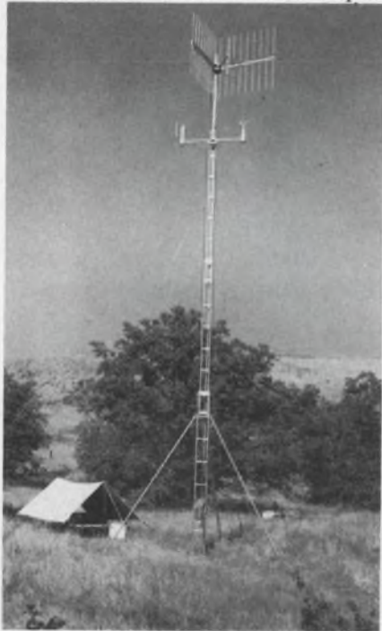
2. Portable field weather station consists of ground electronics and 30-ft tower equipped with meteorological sensors. The station, available from Systron-Donner, contains a control and modulating unit, uhf radio equipment and batteries and is periodically interrogated by a central weather station 25 miles or more away.
