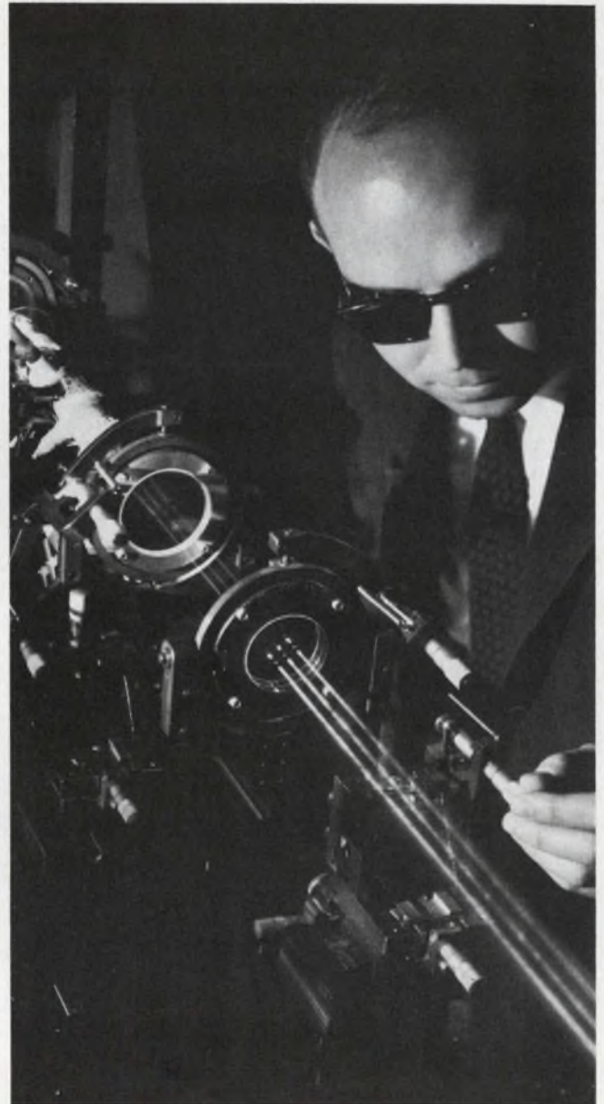
Scanlaser uses electron beam of cathode-ray tube to control laser scanning. Page 33
