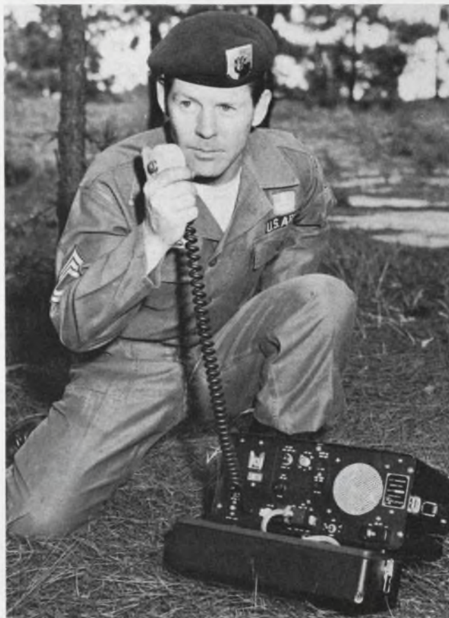
The TR-20 is the base-camp radio used to communicate with the HT-1s carried by Montagnards on patrol. It puts out 20 watts at 30 to 40 MHz and weighs 20 pounds. Sgt. Chambers demonstrates operation.
