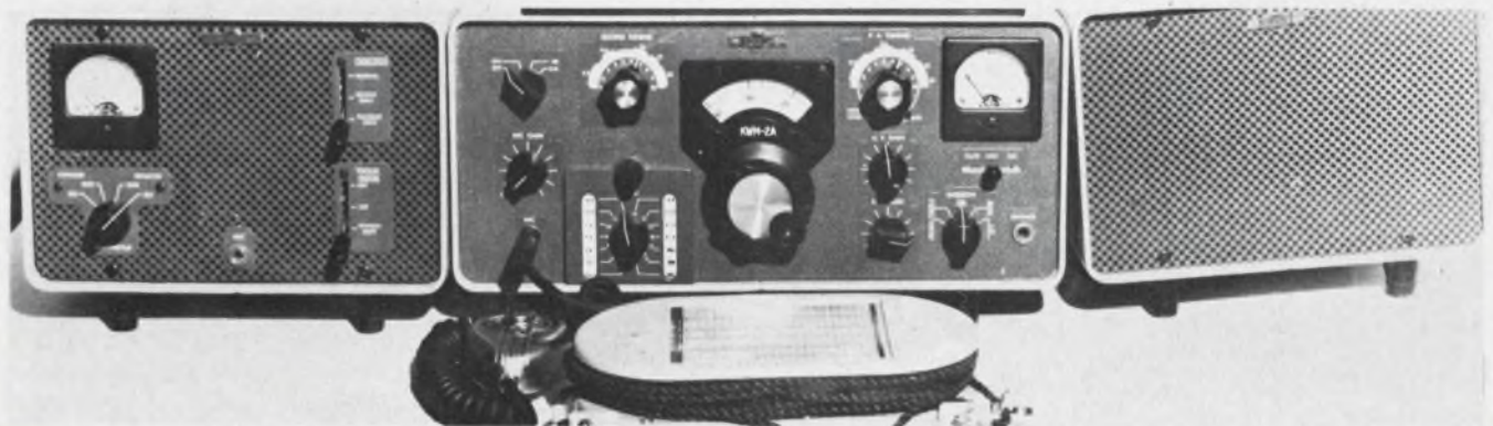
A popular ham radio, Collins KWM-2A was bought off the shelf and since has become the backbone of Special Forces communications in Vietnam. The Green Berets say they can talk to the U.S. almost as easily as to the next
