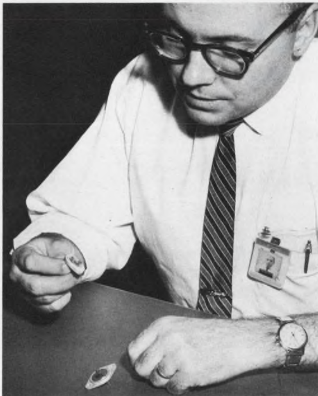
Open-and-shut case of power device mishap. Author Balthasar examines power transistor that failed. Why? Because the prescription for safe operating area wasn't followed and second breakdown occurred.
