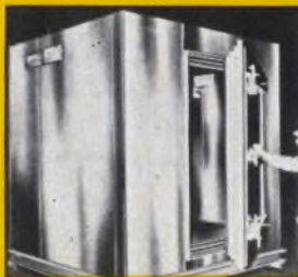
Magnetically Shielded Room
