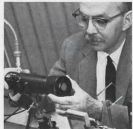
Silicon disk is placed over the aperture of a photodetector housing as an attenuator for laser measurements.
