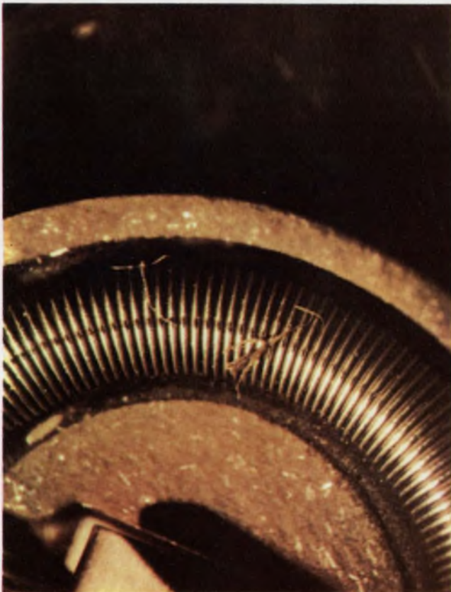
Ordinary lint on a wirewound potentiometer was sufficient to produce noise spikes, illustrating that even the smallest particle can cause trouble.
