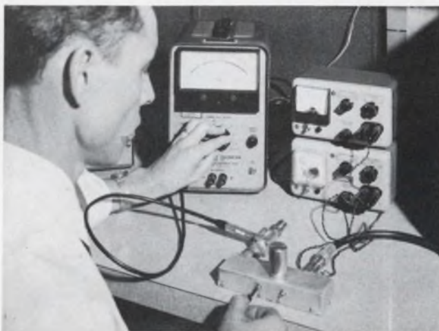
Reaping the benefETs: Author Pierson checks the performance of his FET 500-MHz linear amplifier. For uhf operation, the common-gate mode exhibits good gain and bandwidth, low noise and excellent stability.
