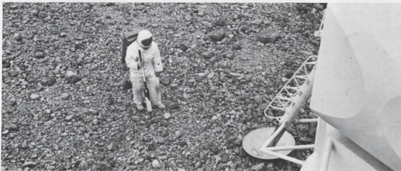
Sweating out a stroll over a simulated lunar landscape, John Slight, test engineer, wears an Apollo pressure suit, a thermal over-garment, and a life-support backpack. A Jacob's staff here aids in walking. He is approaching a full-scale mock-up of the LEM used in simulation studies.
