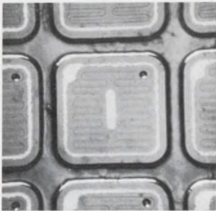
An inside view of the Crystallonics power FET. Each device can handle nine watts.
