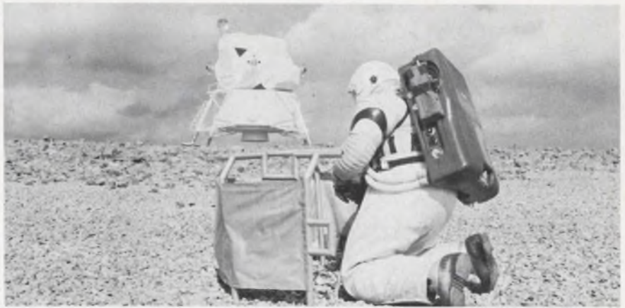
Lunar Topographical Simulation Area provides an eerie setting for tests of the portable life-support backpack and a "lunar walker." The backpack system weighs about 60 pounds on earth, 10 on the moon. The walker helps the astronaut move over the rough terrain in his bulky suit.
