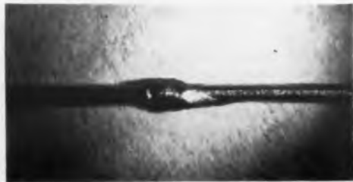
Fig. 2. A collar of gold-tin-lead alloy was formed above the solder level when this gold-clad nickel wire was dipped for 5 sec in a 450 F 60/40 solder bath. The gold was removed from the immersed (right hand) end of the wire during the formation of this collar.
