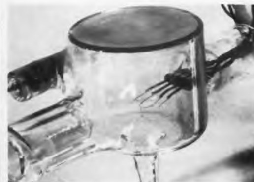
This specially designed tube was used at the National Bureau of Standards for experimental verification of the field emission of electrons from metals.
