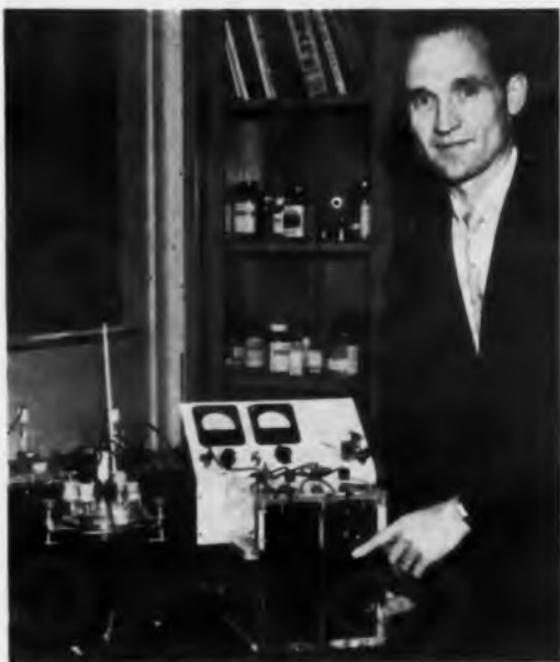
Bacteria culture in the battery cells produces electricity, as illustrated by Dr. Gilson H. Rohrback, president of Magna Products, Inc., Santa Fe Springs, Calif.
