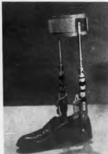
Short leg brace is instrumented with strain gages oriented to permit analysis of the various forces involved in walking with a brace.
