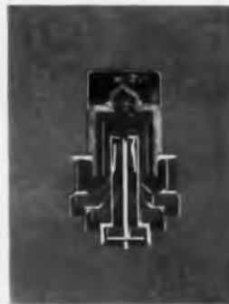
"Cutaway of RCA-7801 showing unitized electrode and terminal construction"
