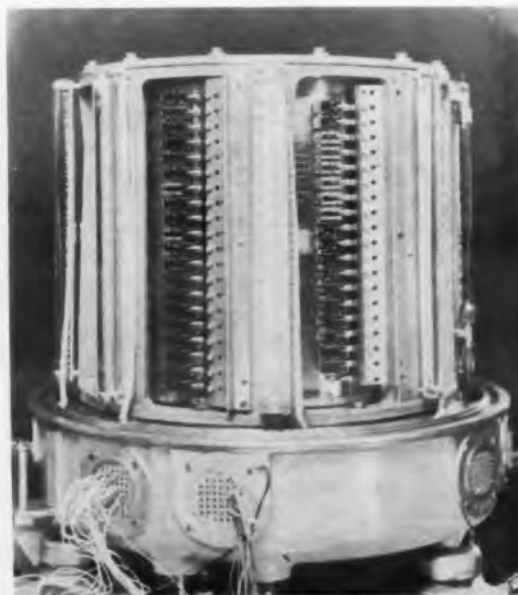
Fig. 5. Magnetic file drum by Laboratory for Electronics, Inc., is only 14 in. high, 15 in. in diameter. It can store 15 million bits with an average access time of 180 msec.
