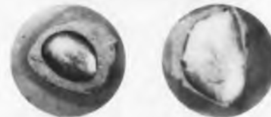
Sample, left, shows ordinary solder. Sample, right, shows ALPHA Cen-Tri-Core Solder's 33 1/3% greater flow.
