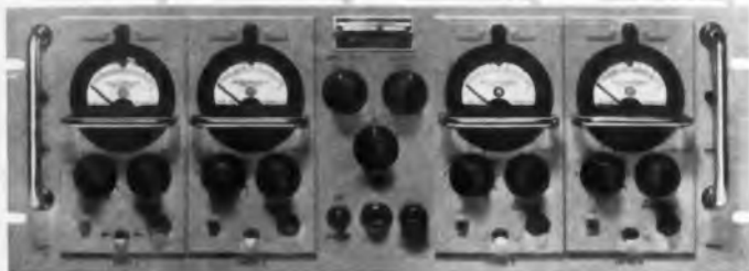
DCA-1000A DIVERSITY COMBINER. COMBINING ACTION IS OBTAINED BY SAMPLING NOISE OUTPUT OF EACH RECEIVER BY MEANS OF HIGH-PASS FILTERS.
