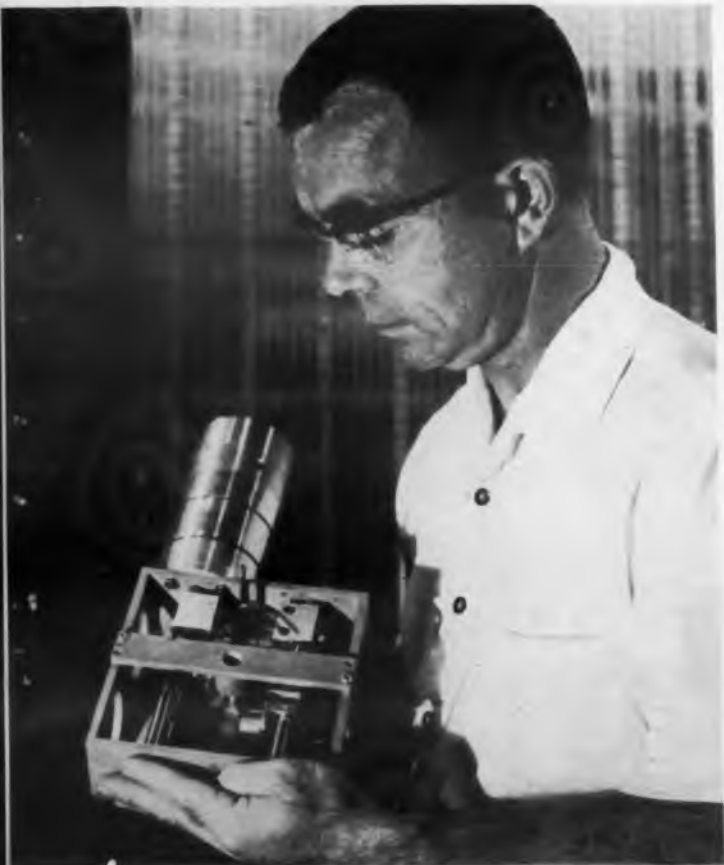
AiResearch engineer holds one of the new air-operated analog computing modules. The 1-ft-long, 4-lb units will sell for $500. Computing will be done by balancing forces from pneumatic inputs acting on pivoted rods. Cylinder extending away from box houses piston which is used for moving the input force along the rod during multiplication.
