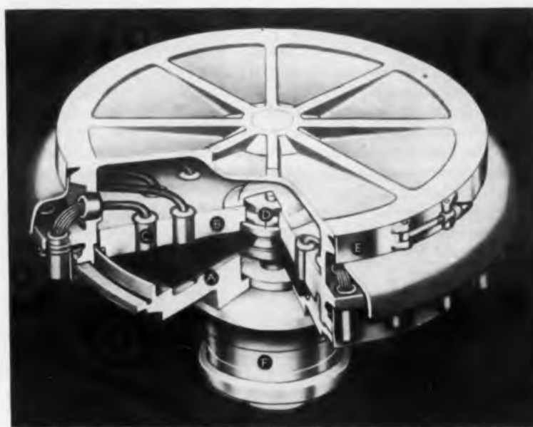
Fig. 7. The BD-500 Bernoulli Disk memory of Laboratory for Electronics, Inc. can store 500,000 bits. In the drawing, the black section (A) represents the flexible Mylar disk. (B) is the stabilizing backplate, (C) is one of the read/write heads, (D) is the backplate bearing cartridge, (E) is a connector ring, and (F) is the drive motor.
