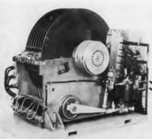
Fig. 9. Multiple disk file made by Bryant Computer Products can have as many as 20 disks.
