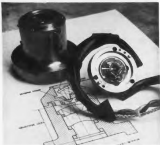
Disassembled Optag pickoff. Arrow indicates nose of sensing prism surrounded by four lead sulfide detectors. A flat-field Schmitt objective lens is housed in metal cylinder at left.
