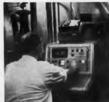
SPACE MEDICINE RESEARCH. In simulated space environment testing, this NLS V34 digital voltmeter is part of a system which detects and records minute changes in body weight, a key factor in determining physiological strain. The unique "No Needless Nines" logic of the V34 permits measurements at pre-selected time intervals with an accuracy of \pm 3 grams within a range of \pm 4,500 grams. AMF's Mechanics Research Division developed the overall system under direction of the Air Force's Aeronautic Systems Division at Wright-Patterson AFB in Ohio.
