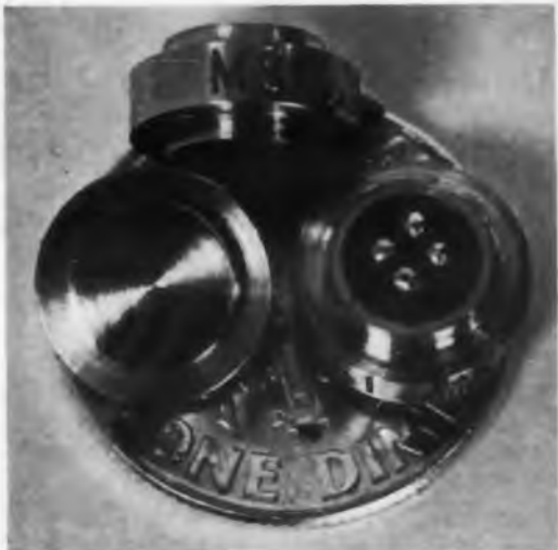
Subminiature pressure transducer marketed by Micro Systems, Inc., contains four silicon filaments as strain sensors, arranged in a Wheatstone bridge. Output is 2 v with a pressure range of 0-100 psia.
