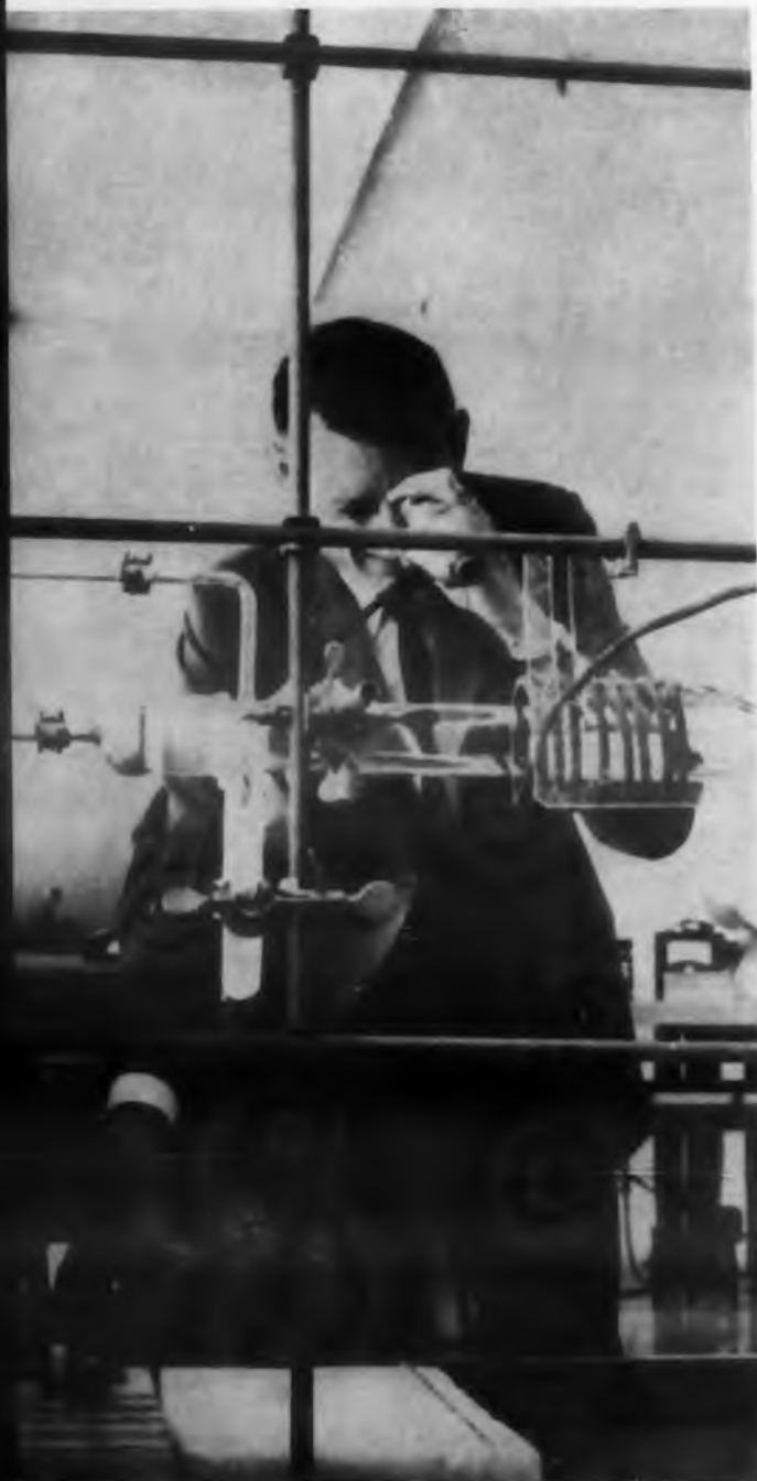
Dash process furnace for epitaxy studies of semiconductors is examined by Dr. Richard Ewing of Shockley Laboratories with a filter viewer which provides magnification of the phenomena.
