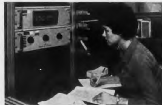
CHECKOUT OF MISSILE COMPONENTS. An M24 checks electronic components at Autonetics, a division of North American Aviation, Inc., as part of the High Reliability Program for Minuteman ICBM. The operator is shown measuring resistance. By turning a front panel knob on the M24, she can also measure DC voltage or DC voltage ratio.
