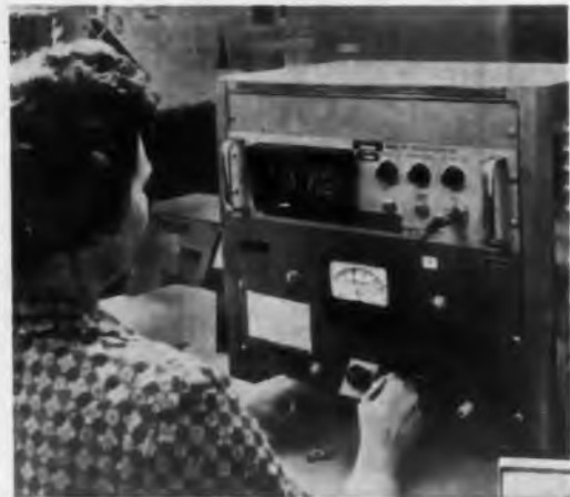
QUALITY CONTROL OF ELECTRONIC COMPONENTS. More than 50 NLS 481 digital voltmeters are used in the Quality Assurance Program at the Semiconductor Components Division of Texas Instruments Incorporated. The instrument pictured is measuring breakdown voltages of high-reliability germanium switching devices.
