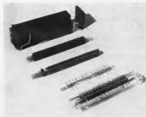
Fig. 1. Various stages of assembly for a logic stick designed for the Polaris computer.
