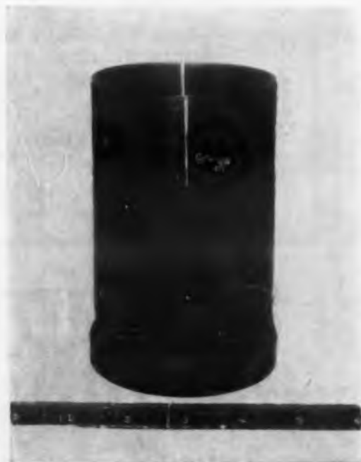
Plastic sabot fits over projectile inside the gun and breaks away upon firing.
