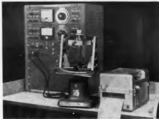
In this simple bench set-up, the 906 Visicorder is at right. Between it and the control panel is the Scorsby table on which the gyro is mounted, ready for test.
