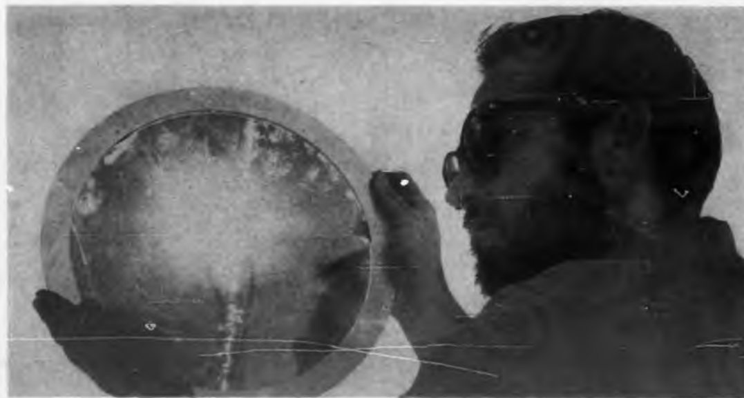
Light collector for Socom is inspected by scientist of Electro Optical Systems, Inc. The company is developing space optics said to weigh less than 0.4 lb per sq ft. Mirrors can be either rigid or foldable.
