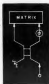
Fig. 9. Hybrid connected to form cosine taper illumination beam. Phase shifter adjusts the phase center of one matrix beam to coincide with the phase center of the second matrix beam.
