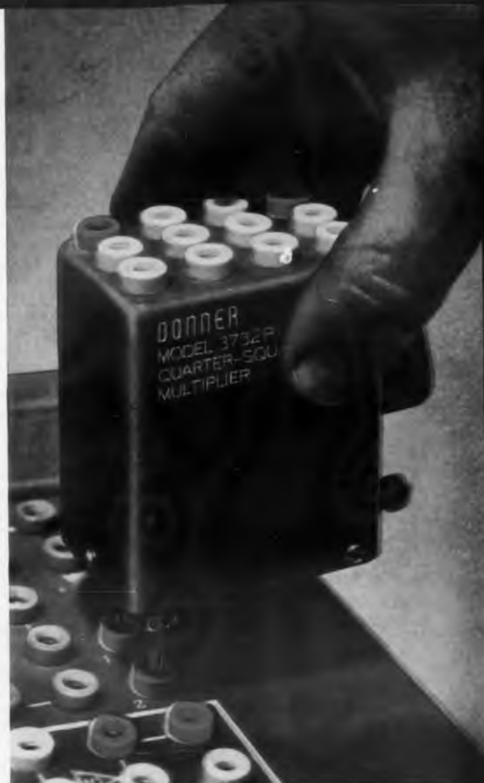
Model 3732 electronic multiplier is available without enclosure for panel mounting or as a single printed card for inclusion in your system. The unit is also available with up to three solid state multipliers on a 3 1/2" x 19" panel for rack mounting.
