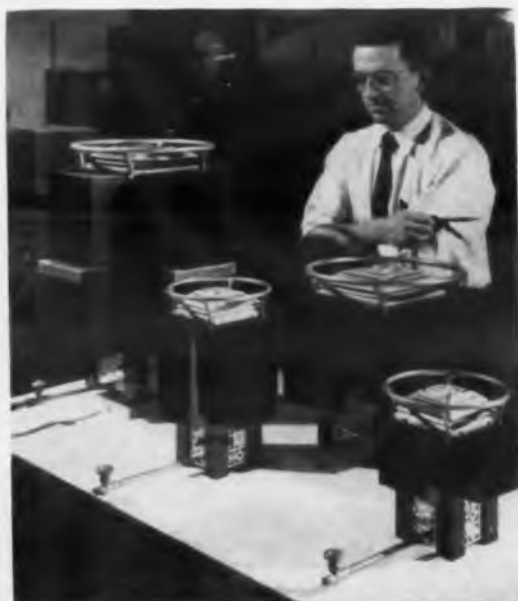
Westinghouse engineer checks over 5-, 10-, 50-, and 100-w thermoelectric generators now commercially available, on a prototype basis, from the company. Price ranges from $1,700 to $6,000.
