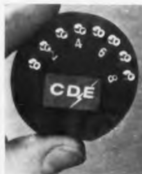
Mica Capacitor Network Is 0.190 In. Thick 523
