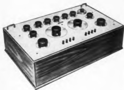
DC Vernier Potentiometer Has Accuracy of \pm 0.001\%
