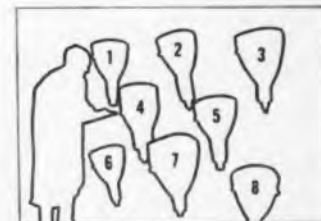
1. 12AKP7, radar tube. 2. Z-4760, 2-gun, 12". 3. Z-4718, low drive, 12". 4. Z-4778, 2-gun with integral magnetic shield, 12". 5. Z-4701, minimum deflection defocusing, 12". 6. 12 ANP-14, high performance radar. 7. GL-4623, 16" electrostatic deflection. 8. Z-4652, tetrode tube design, 12".
