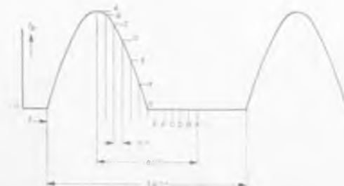
Fig. 1. A periodic symmetrical waveform, typical of an rf amplifier plate current pulse, is divided into thirteen 15-deg segments for harmonic analysis.
