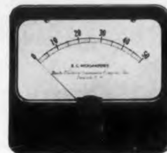
MODEL 16 - BAKELITE - FLUSH 4 1/2" x 3 1/8"
