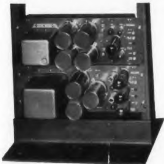
MR-40 microwave transceiver for 12 Gc is klystron-driven. Manufacturer predicts rapid growth of microwave business radio as result of new FCC policy.
