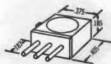
THE MODEL 50 3/8" square, 3/16" high, and weighing 1 gram, the Model 50 is available in standard resistances of 50 ohms to 20K ohms.
