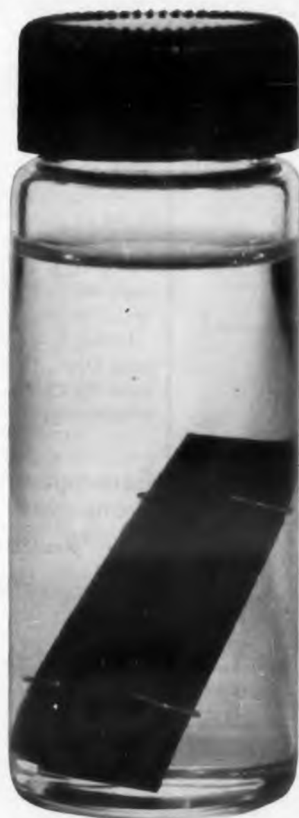
"FREON" SOLVENT left this acrylic resin and metal unharmed after prolonged exposure.
