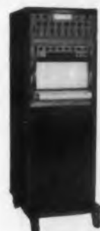
Simplified 6- or 8-channel system, 5 volts full scale.
