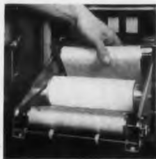
Easy threading of chart paper to internal take-up roll for data storage.
