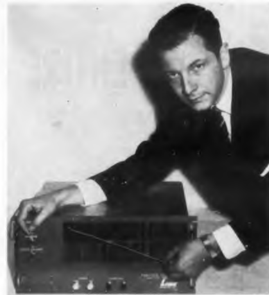
Analog function generator fits in a 19-in. rack, provides a voltage z = f(x, y) with \pm 1 per cent accuracy.
