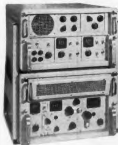
Single-Sideband Receiver, Model AN/WRR-2, developed by National Company, Inc. for U. S. Navy installations, used Hermes SSB Crystal Filters, Models 869U and 869L.
