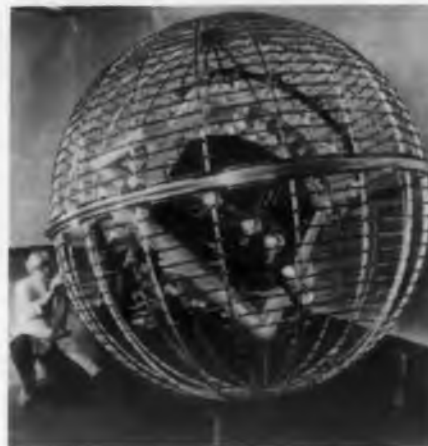
Tiros II is mounted in a spherical cage for test of new magnetic orientation-control system which adjusts axis tilt.
