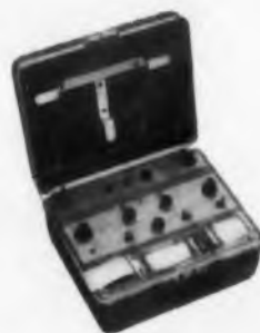
1-channel, 21 lb. portables — Model 299 for general purpose DC recording, Model 301 for AC strain gage recording.
