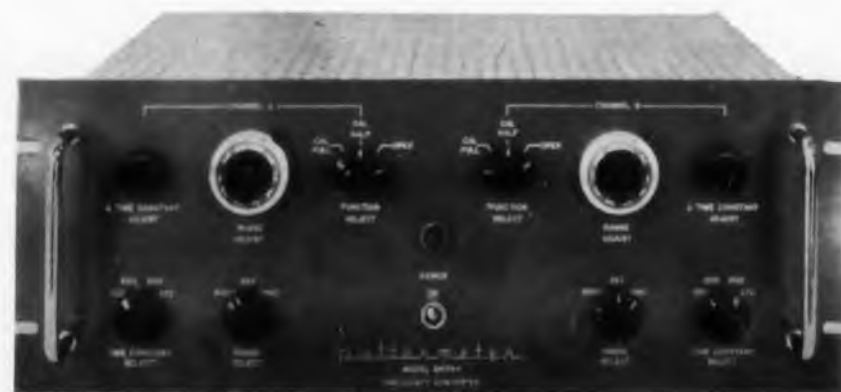
Frequency-To-Analog Converter 1s Accurate To 0.1% At Up To 10 Kc
