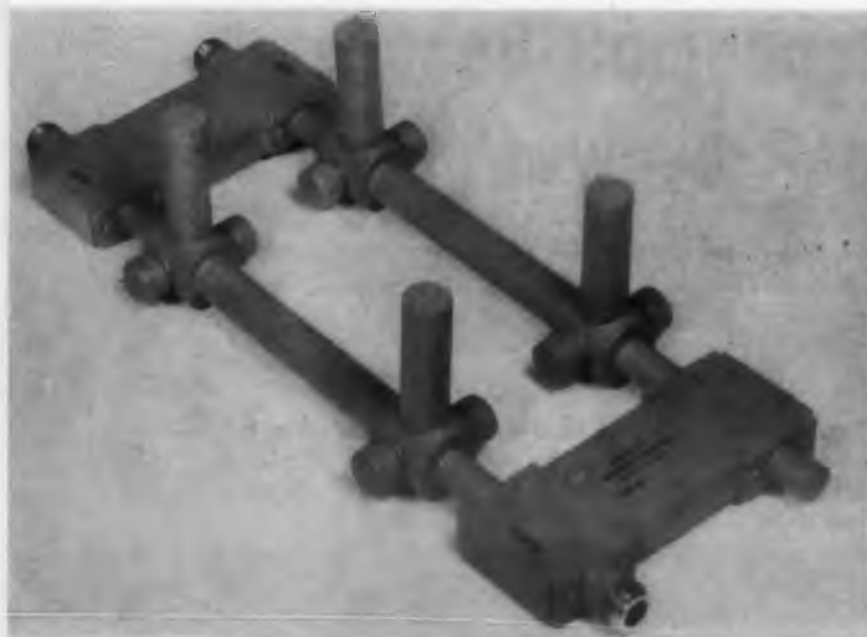
Fig. 4. Solid state "tinkertoy" duplexer includes balanced limiters, enabling it to handle 10-kw peaks while recovering in 10 nsec.
