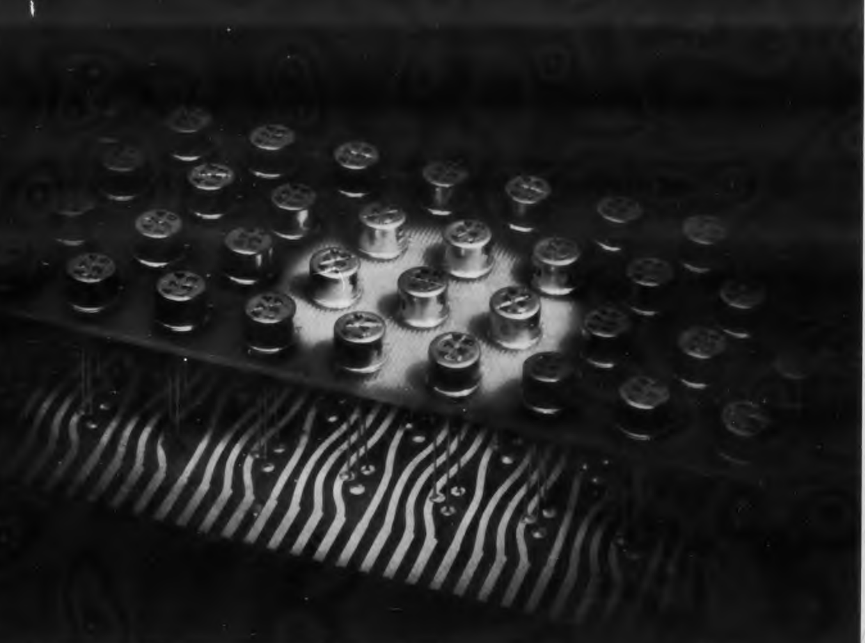
Carrier-matrix board designed by Autonetics tests groups of 100 Fairchild Transistors simultaneously
