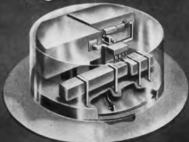
1. New surface-wave Luneberg lens concept for 1-inch-thick antenna provides 360° look in single sweep.
