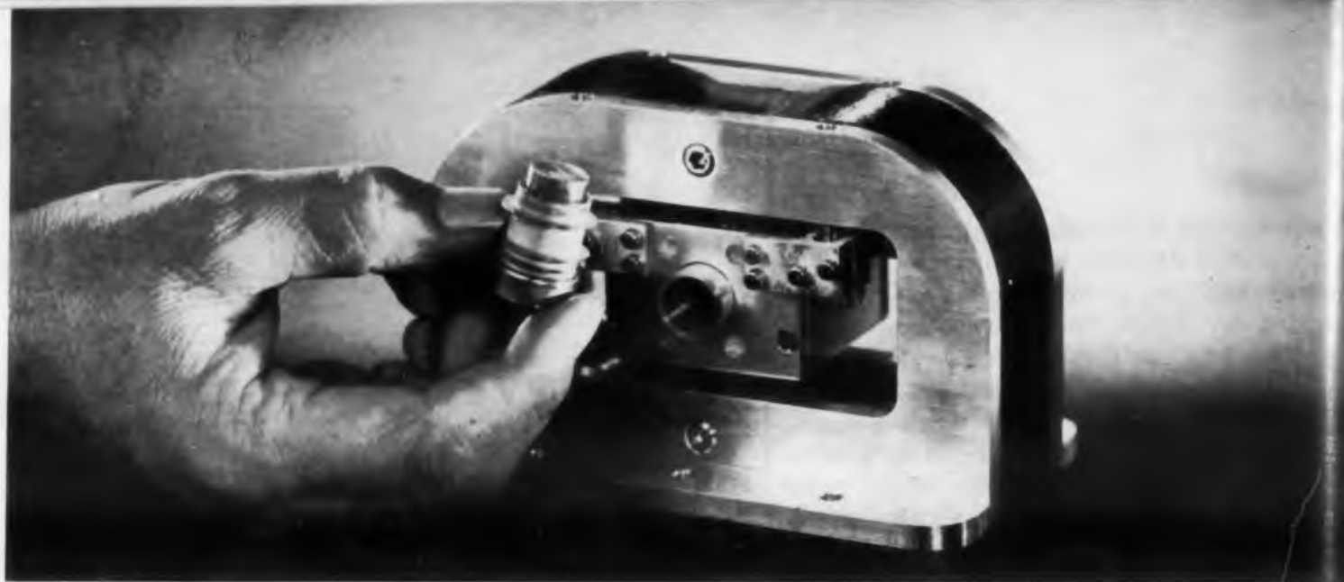
Fig. 1. 100 mw of electronically swept output over 400- to 1,200-mc range available from new EIMAC X-747 VTM. Tests so far indicate linearity better than 1 part in 1,000.
