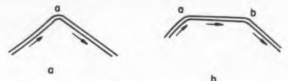
Fig. 2. Straight waveguides, bent in one or two places, radiate in the sections near the bends.
