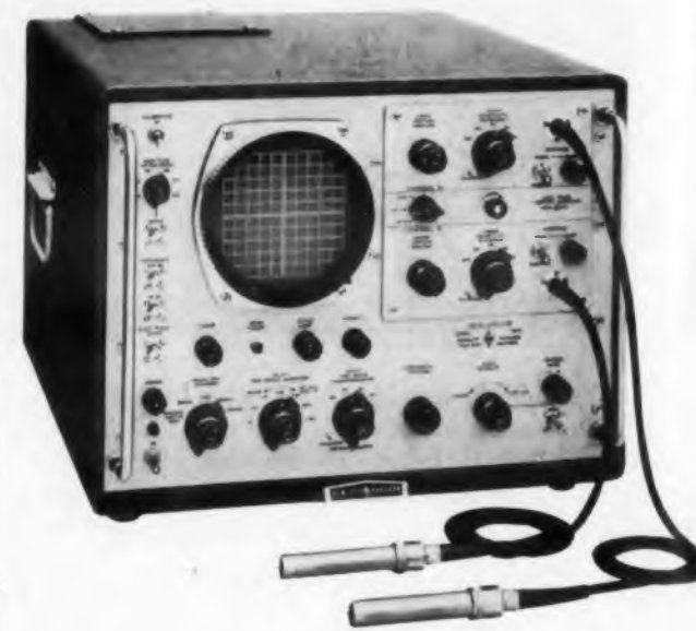
Fig. 6. Hewlett-Packard Model 185A sampling oscilloscope faithfully displays sub-nanosecond pulses with its DC-1000 megacycle bandwidth. High sensitivity of 3 mv per cm permits even small reflections from vhf elements to be analyzed with ease using pulse reflection techniques.
