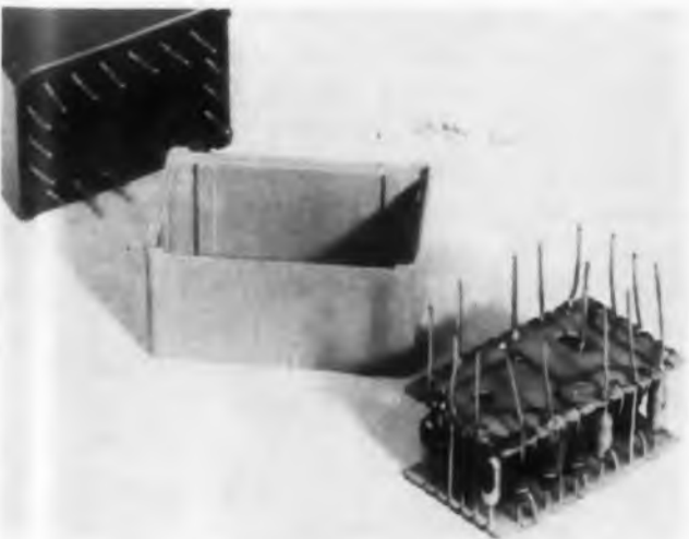
Fig. 4. Component leads can be left to extend straight out of the shell after encapsulation.
