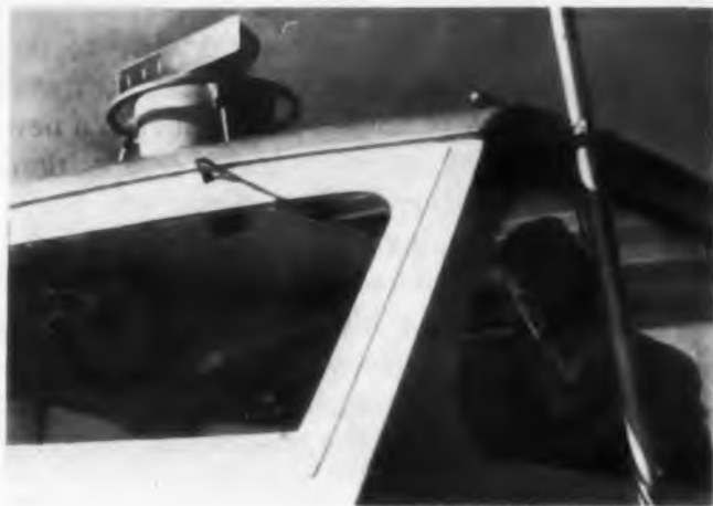
Fig. 4. One of the smallest and most inexpensive microwave systems, this Sperry Radar 5 is a safety boon to small-boat operators.
