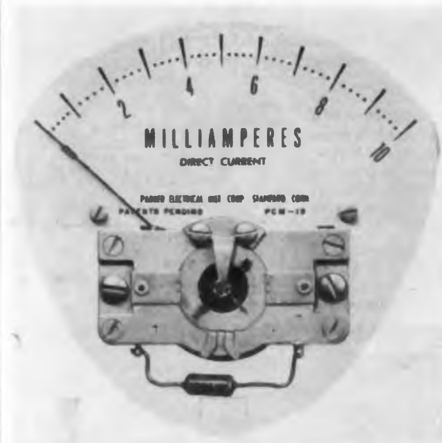
Paper-thin meter rotor consists of printed coils on anodized aluminum base.
