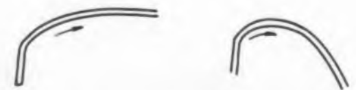
Fig. 4. Slightly curved shapes produce a co-secant-shaped directivity pattern.
