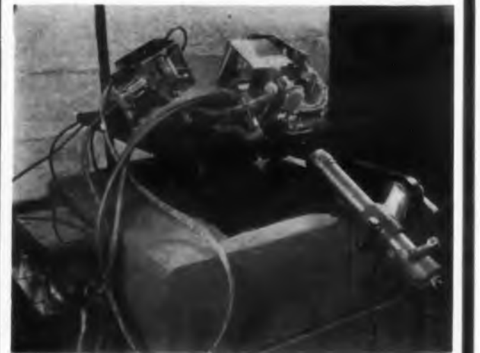
Tom Cat III infrared horizon sensor being aligned at General Electric is part of the company's Tom Cat series of sensors. Computer box is mounted to left and below the three sensor heads, which are in aluminum housings.
