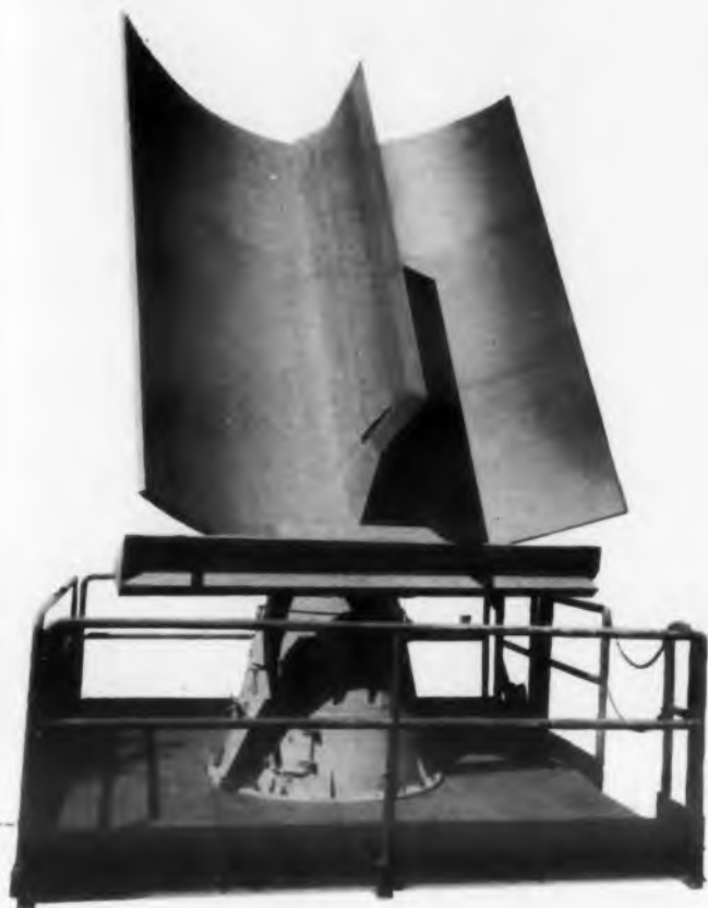
Fig. 1. Line source and parabolic cylinder allow electronic scanning to be effected by change in frequency.
