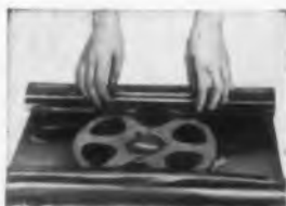
Thin pliable foil wraps easily around magnetic tape, maintaining original recorded fidelity.
