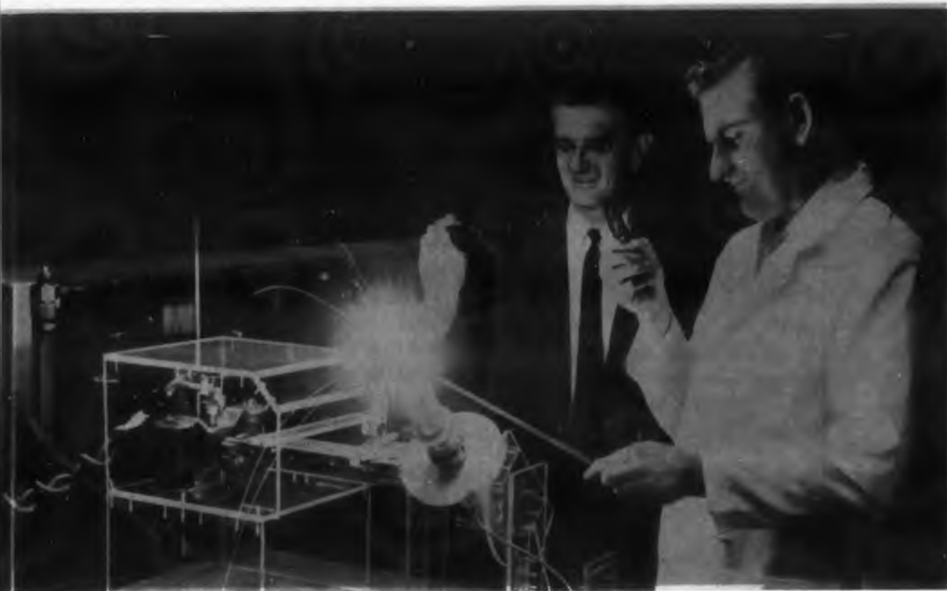
Fig. 1. A plasma-microwave torch, capable of melting a steel rod without itself becoming warm, was recently announced by Amperex.
