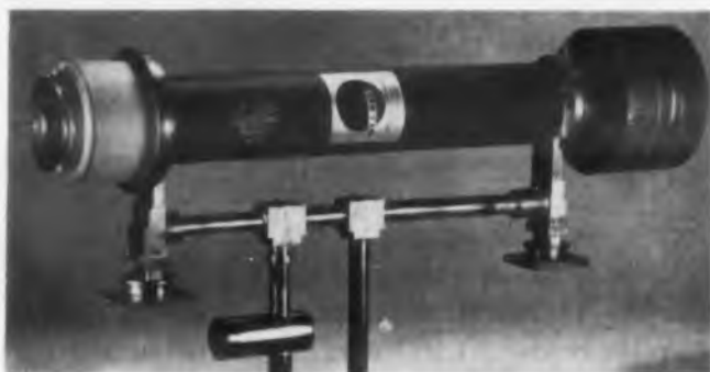
Fig. 4. In just three years, Varian's 20-kw VA-849 klystron has increased available power an order of magnitude in the 7.125 to 8.5 Gc range.
