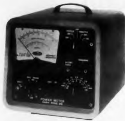
Fig. 3. This Narda Model 440A power bridge is fully transistorized allowing it to operate from a rechargeable nicad battery. This eliminates drift caused by changes in bolometer bias current and provides for a fully portable rf power measurement.
