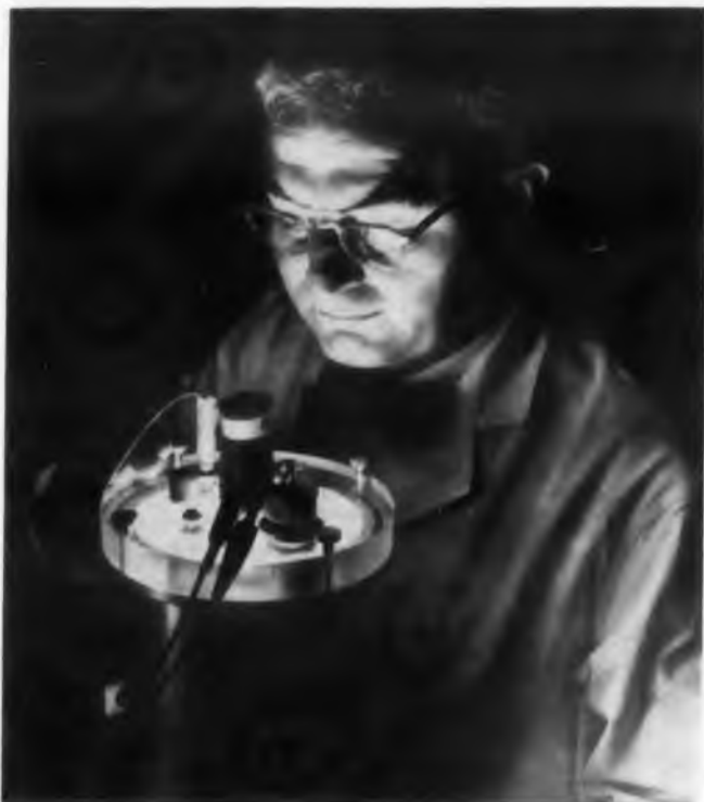
A krypton-86 lamp in its liquid-nitrogen bath is adjusted by a National Bureau of Standards scientist. The wavelength of the orange-red light emitted by the lamp has been adopted as the international standard of length. The lamp is operated at the triple point of liquid nitrogen, 63 K, to increase the stability of the standard wavelength.
