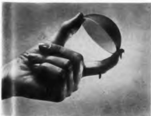
Defense Dome: Irtran forms a dome for the nose of an infrared-missile. It transmits radiation efficiently up to 8 microns in the infrared.
