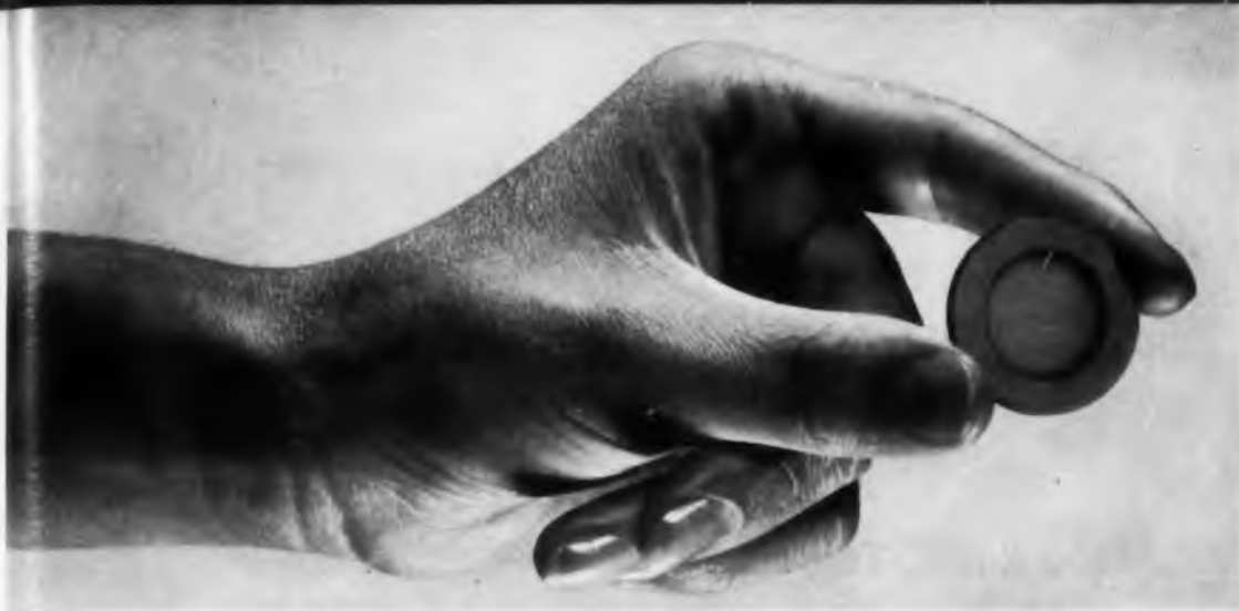
Guidance Disk: Partially plated disk of Irtran material has been polished with methods normally used for glass. It is designed to serve as one of a pair of missile "eyes."
