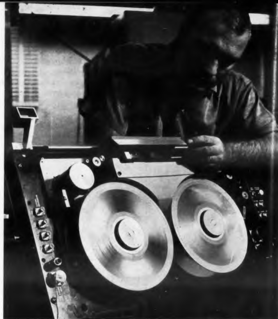
Engineer checks rotating head assembly on airborne wideband recorder.
