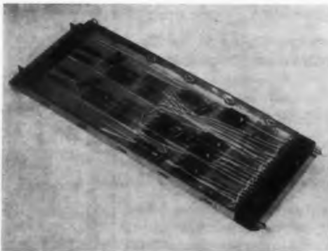
Female connector (more likely to fail than male) is mounted on plug-in card in Univac III and Larc computers rather than in equipment rack.
