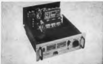
"Flip Top Box" Permits Accessibility For Maintenance
