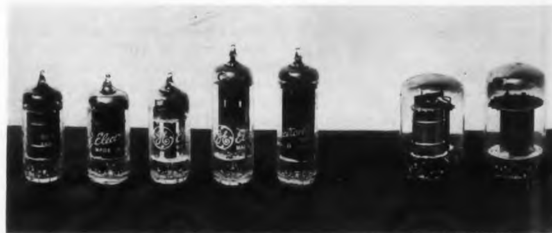
Two compactrons (right) replace five conventional miniature tubes (left) in a table-model radio. A TV set would require 10 compactrons.
