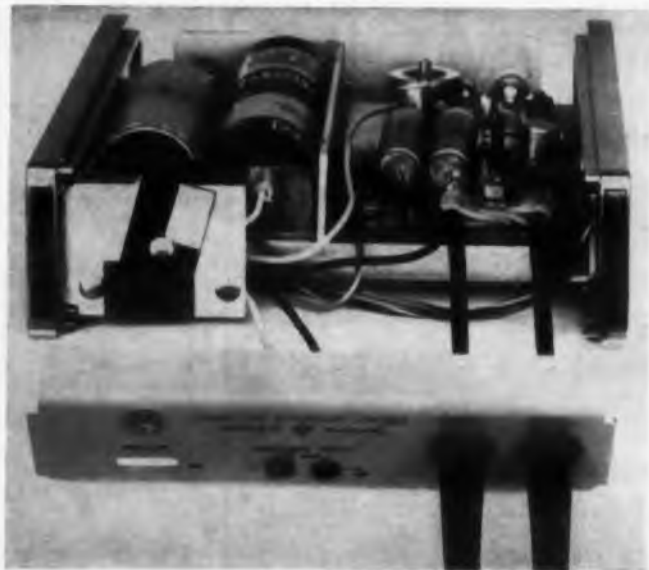
Light-reflecting red tape, pivoted into position by on-off switch, serves as powerless pilot lamp.
