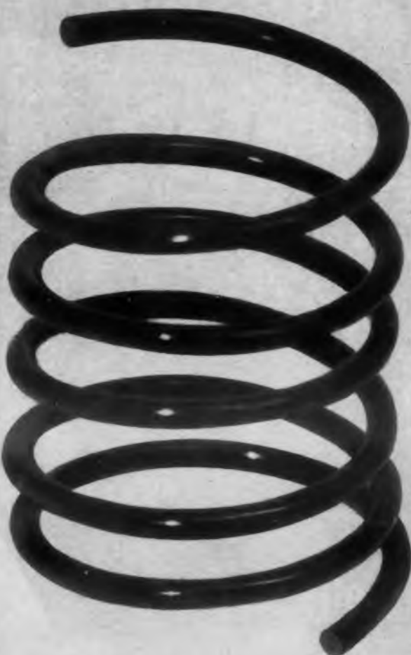
This magnet wire was exposed to "Freon" solvent liquid. The "Glyptal" coating on this wire is completely unaffected by "Freon"-TF.
