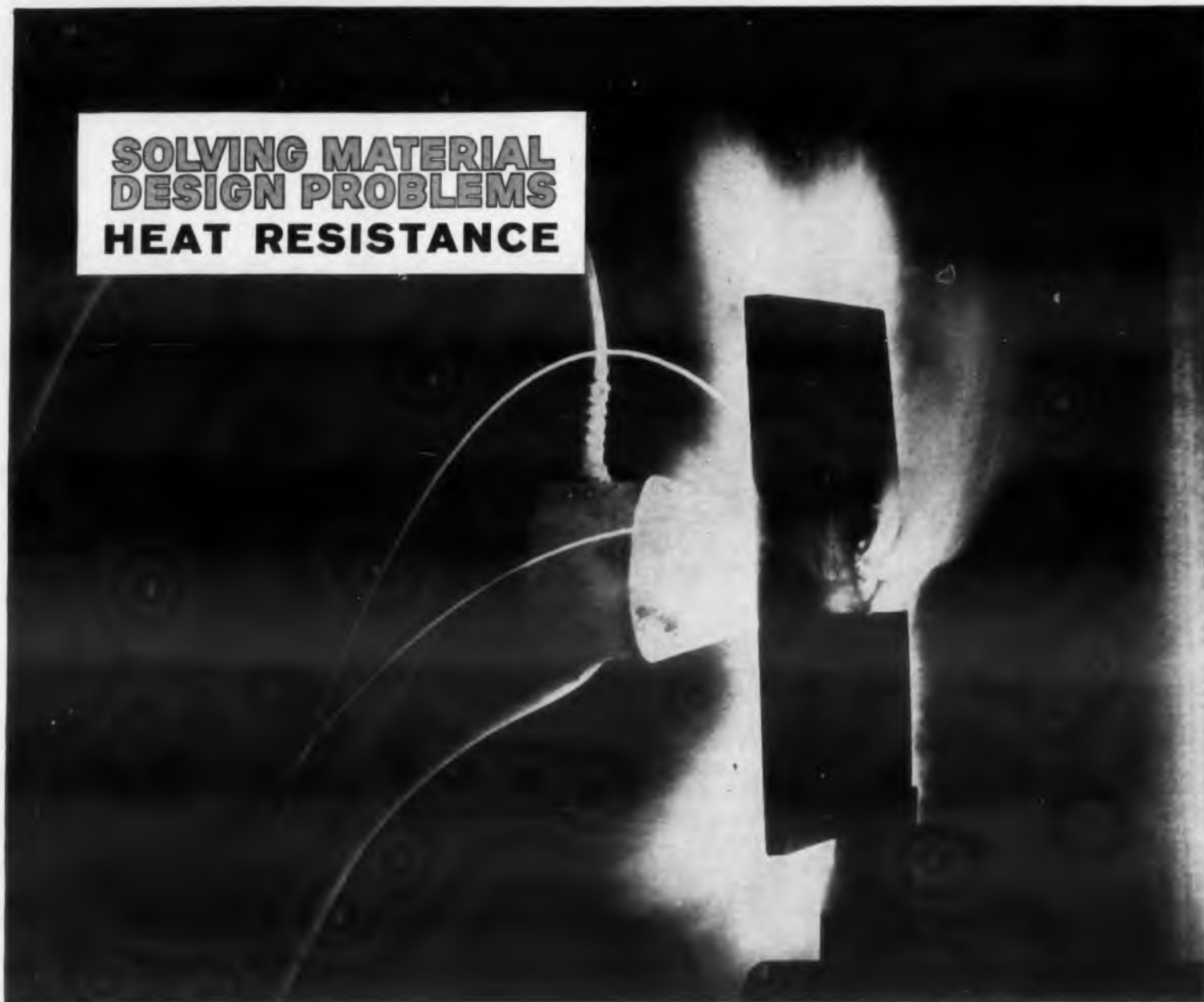
A 5000° flame takes ten minutes to penetrate a one-quarter inch piece of CDF's new Dilecto RD-105 laminate. The same thickness of cold-rolled steel is pierced in less than forty seconds.
