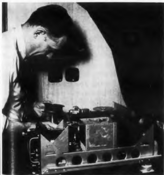
Magnetic tape flight recorder gets final check aboard a Minneapolis-Honeywell airplane. An engineer installs a spool of magnetic tape which will record for 150 hours. The M-H recorder is capable of monitoring as many as 65 different variables.
