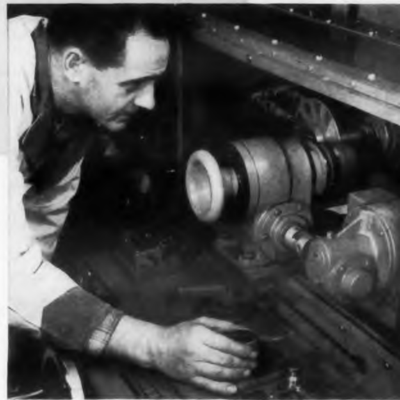
Large silicon crystal being wafered on an MTA-7. Wafers .030" thick are being cut at 1 sq. in. per min. with parallelism between .001" and .002".
