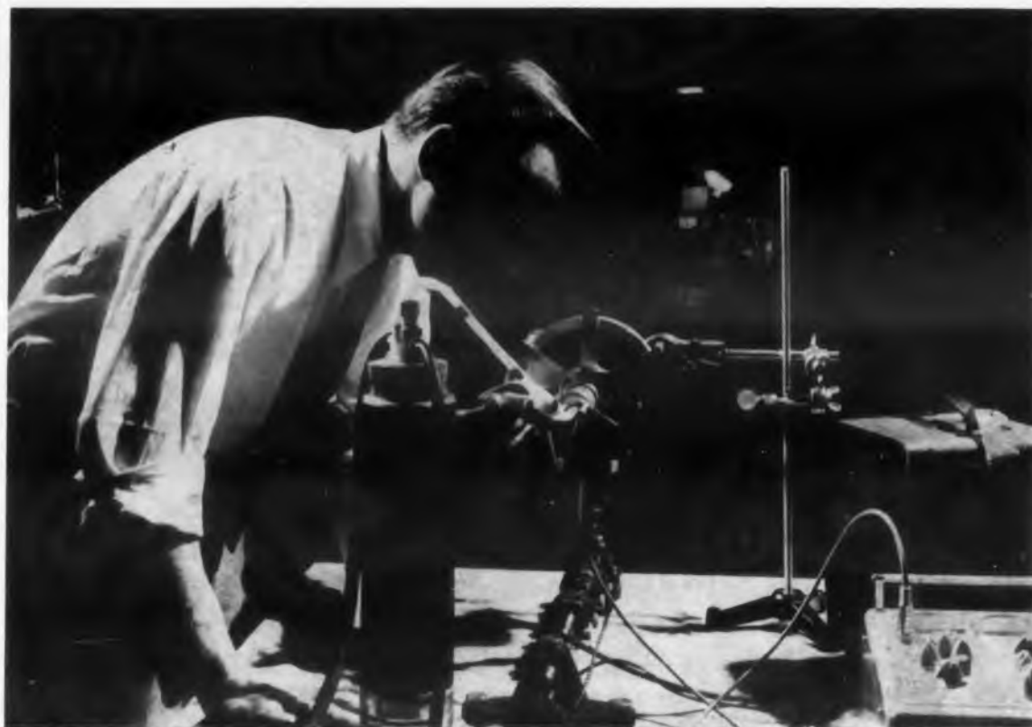
In radiation room at Sperry Gyroscope, Great Neck, N. Y., engineers test new infrared detection device. Eighty-six-ft long tunnel is painted completely black.
