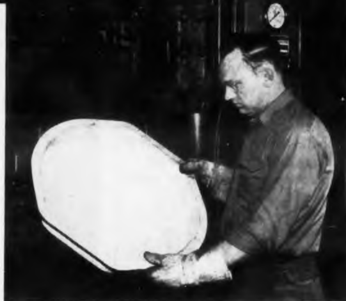
DRAWING. This gyro cover is drawn in a single operation. It replaces a part which consisted of welded components.
