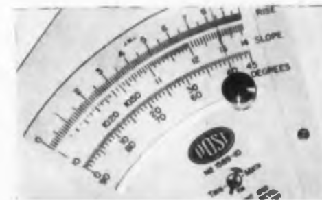
An indicated angle of 40 degrees on the TrigMatk (1589) shows directly that the Rise is 8.4 to the base of 10.
