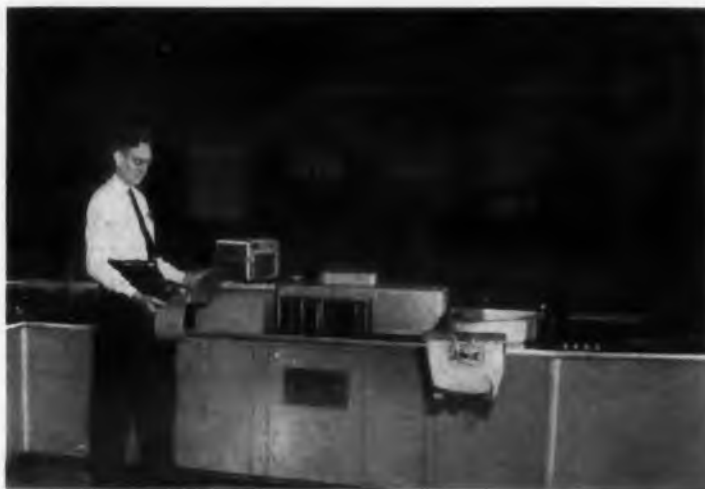
Milton Stovall, Emerson Project Engineer, uses the Visicorder to measure roller bounce caused by various letter thicknesses, and the consistency of letter speed through the new Emerson Automatic Mail Cancelling and Facing Machine.
