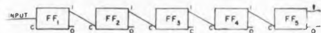
Fig. 1. Flip-flop 5 is triggered only after the first four flip-flops have been reset from 1 to zero.
