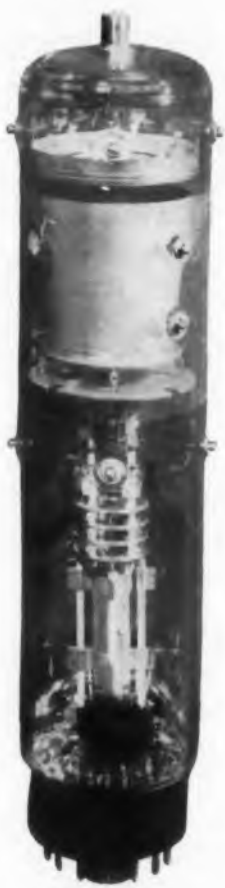
Fig. 1. Photograph of a barrier-grid tube. Sixteen thousand bits of temporary information can be stored here.
