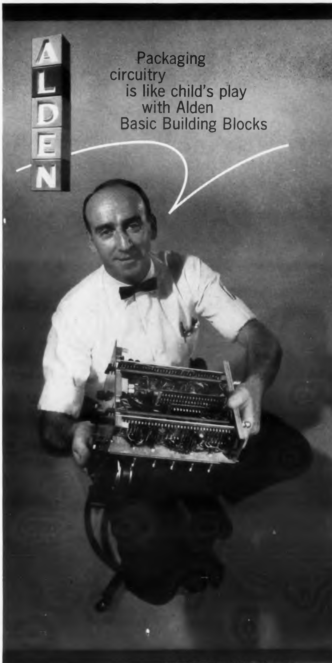
The Alden Basic Plug-in Chassis — with circuitry arranged in space-saving vertical planes for easy servicing, a typical chassis plugs in, locks, ejects with a half turn of the wrist.
