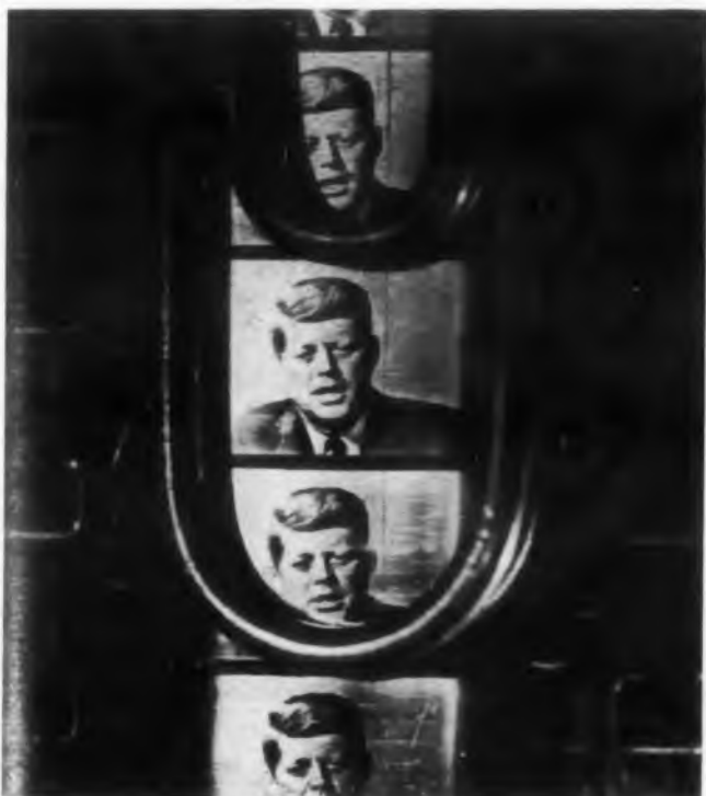
Frames of film produced by experimental model of thermoplastic recorder are about width of paper clip. This film was made by feeding signal directly from TV set if stage to recorder.
