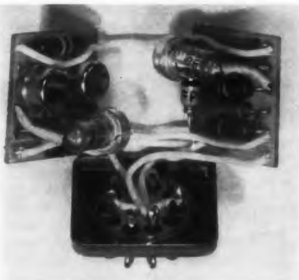
Wired terminal boards of the timing module prior to encapsulation in polyurethane foam.
