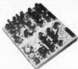
Plug-in modular construction—mechanically arranged for easy access or replacement.
