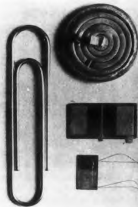
These working molelectronic devices were displayed in Washington by Westinghouse last month: (top to bottom) an audio amplifier, a free-running multivibrator, and a two-stage video amplifier.
