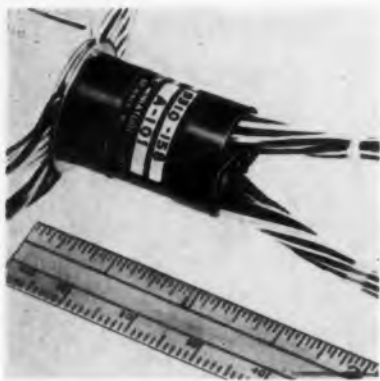
Slip Ring And Brush Assembly Measures 0.982 x 0.624 in.
