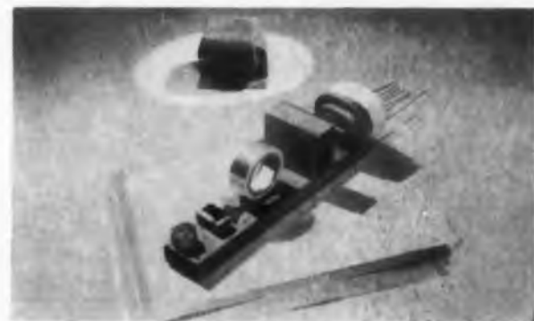
TRANSFORMER CORE TUBE AND LAYER INSULATION
