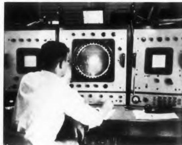
Weather Bureau S-band radar can be switched to X or C band without changing complete waveguide run.
