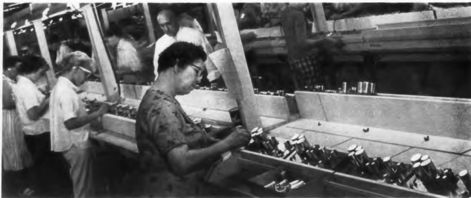
Fig. 4. Kin Tel moves assemblers past stationary parts, cuts learning time to zero.
