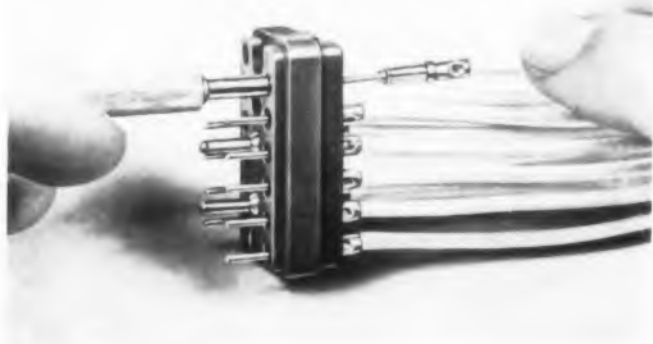
Fig. 17. Burndy's Hyfen connectors allow individual or gang connect or disconnect. The simple extraction tool is used for individual disconnect.
