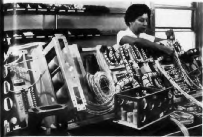
Fig. 6. Worker prefabricates cable harness on wooden dummy of equipment. After harnessing is complete, cables are removed and installed in final equipment.
