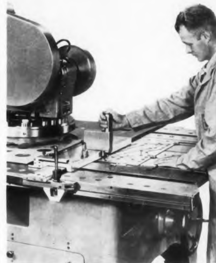
Fig. 5. Operator positions material by following a template on this Wiedemann turret punch press.
