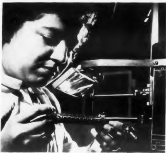
Fig. 14. Raytheon's Weld-power Control applied to solidly packed circuit "sticks."
