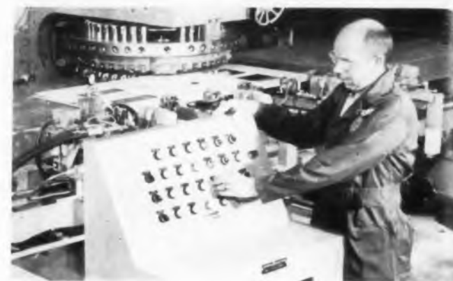
Fig. 6. General Electric's automatic positioning control combines with the power of this Wiedemann press to provide great production speed and flexibility.
