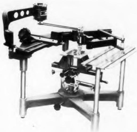
Fig. 12. The new Hermes Engravograph can be used for marking or for deeper cutting applications.
