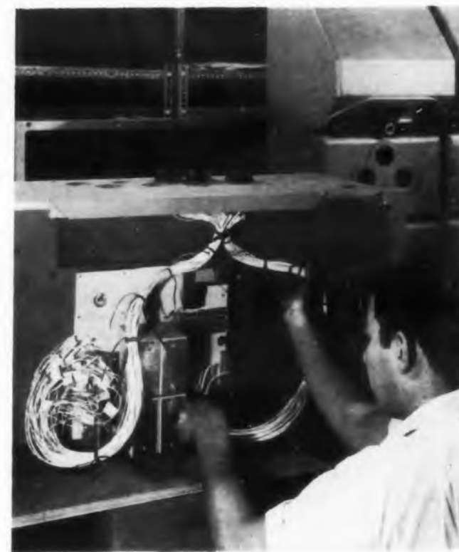
Fig. 5. At Librascope, wooden mockups of equipment are used to lay out wiring prior to actual production.
