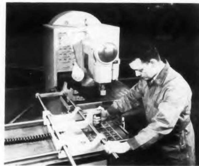
Fig. 7. This Wales-Strippit Fabricator, with an auxiliary Duplicator, follows a template to provide a wide variety of precisely positioned holes.
