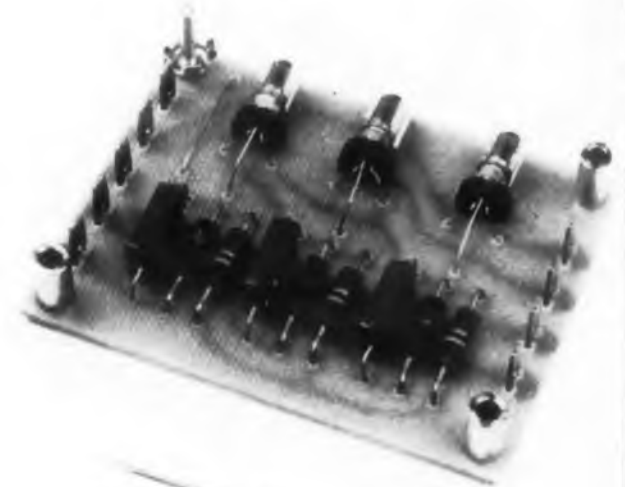
Fig. 2. This single-element card is one of the bricks Sylvania used in building MOBIDIC.
