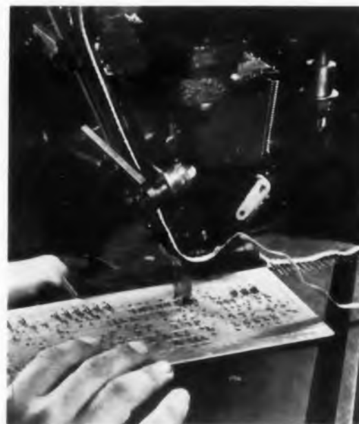
Fig. 2. Dynasert machines cut leads, bend them to fit holes in the circuit board, insert components, and crimp the leads.
