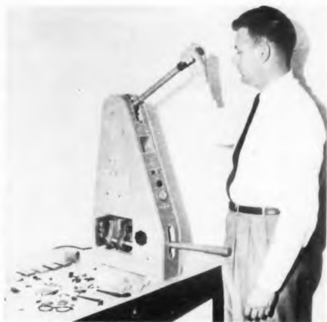
Fig. 13. Hinchman's Unex Jet Molder uses interchangeable injection cylinders and dies.
