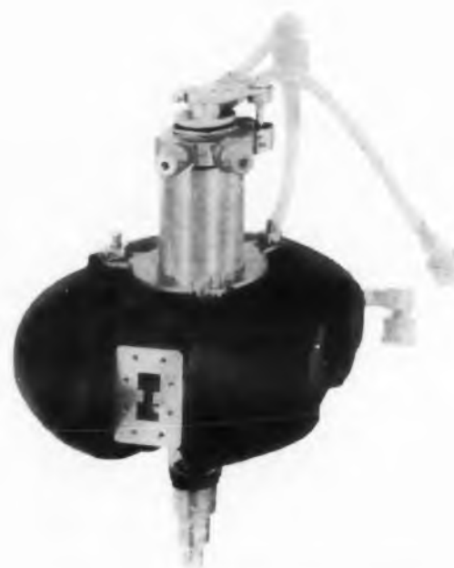
Tunable Barratron tube supplies broad-band white noise.
