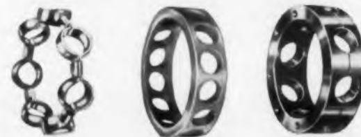
Three varieties of retainers available to you in Fafnir precision instrument ball bearings. From left: ribbon-type steel (for low torque), composition (for high speeds), and iron-silicon-bronze (for high-speed, high-temperature applications).
