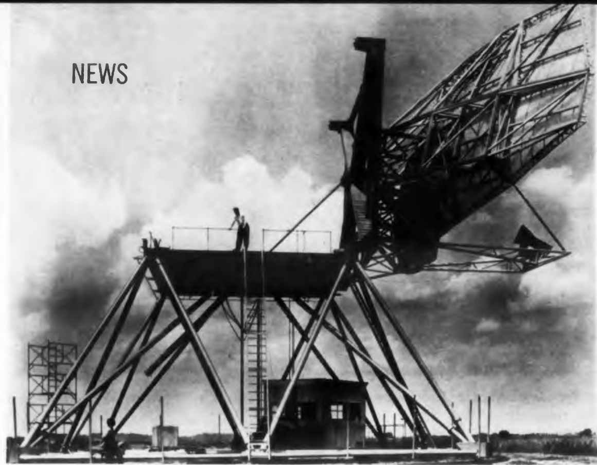
60-foot DEW-line radar antenna undergoing trials at test range of ITE Circuit Breaker Co. near Philadelphia. Dish is mounted on rotatable frame.
