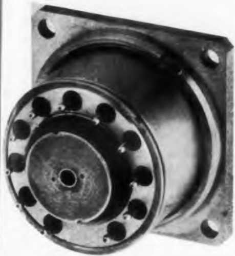
Linear accelerometer (shown almost twice actual size) has unusual resistance to shock and vibration.
