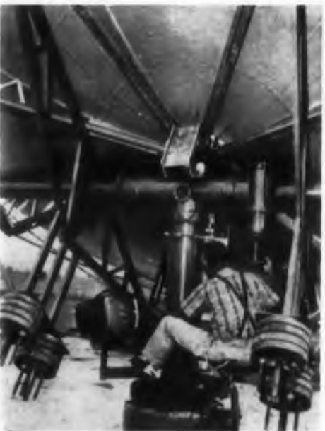
28-foot dish at the University of Texas has picked up moon-bounce signals originating in Great Britain.
