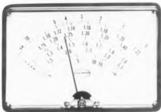
VSWR at any single frequency is indicated on the Ratio-Scan front panel meter.
