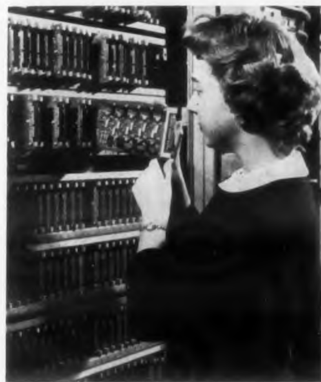
Printed circuit board is inserted into a GE Fire Control System computer, just one of the high-precision instruments installed aboard the test ship U.S.S. Observation Island under the Polaris program.
