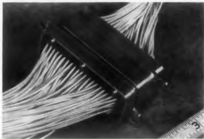
Fig. 6. Contacts on this rack and panel connector are gold-plated for protection against corrosion.
