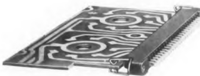
Fig. 2. Spring latch dogs on these P-C receptacles insure vibration-proof mounting of circuit boards.
