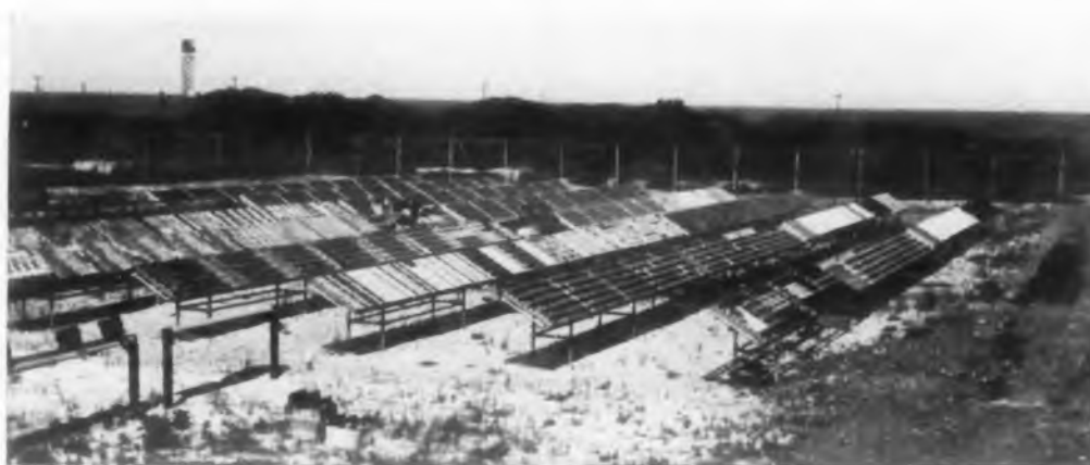
EXPOSURE TESTS on many assembly protection methods and new finishing developments are constantly in progress on these seaside test racks (International Nickel Test Station, Kure Beach).
