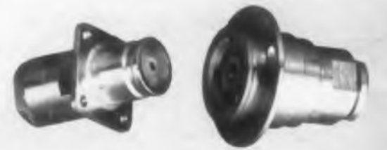
Fig. 3. Captivated center pins, which are built into the rf connector, prevent dielectric creepage from causing discontinuities in the center contact.
