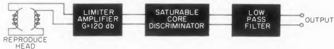
Fig. 4. Fm reproduce discriminator needs large signal amplification and limiting because of fluctuations of output from tape recorder head. This is a standard problem in recorders due to tape, head-to-tape contact and dust.
