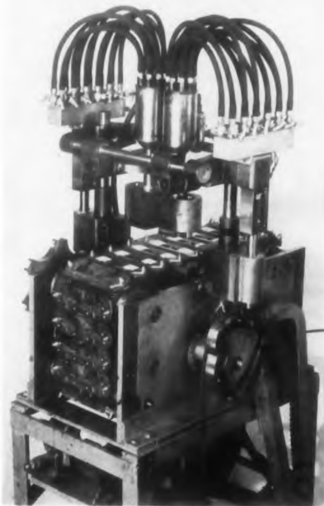
Fig. 5. Injection molding resistor printing machine. Conveyor pauses under the printing head.
