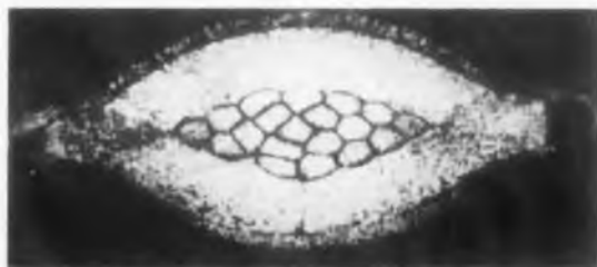
Fig. 1. Good conduction and reliability in a solderless connection depends on the deformation of the wires. In the cross-sectional photograph the compression-type connection is shown.
