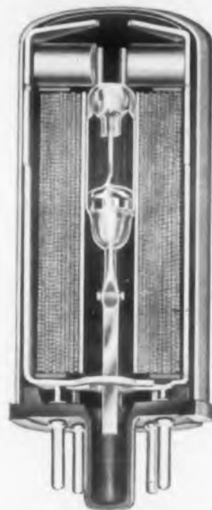
Cutaway view of a CLARE Type HGS Relay. Mercury-wetted contact switch is sealed in glass and surrounded by the operating coil. Biasing magnets are attached to the upper ends of the side plates.
