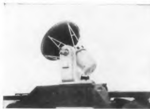
NIKE GROUND GUIDANCE—Large magnesium assemblies are easily and effectively protected by standard finishing methods.
