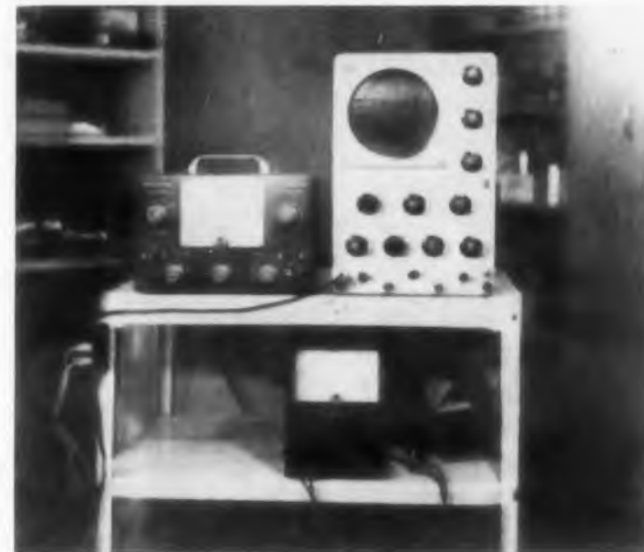
Fig. 1. Utility cart for instruments can be wheeled to bench. Lower racks can be used for temporary storage of equipment not in use.
