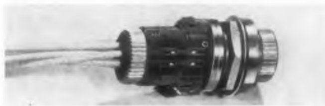
Fig. 2. Cut-away view of the taper pin connector.
