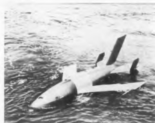
RYAN FIREBEE, with 75% of its exterior surface magnesium, has withstood repeated dunkings in the ocean with no adverse effects. The reason—Ryan applied the proper protective measures.
