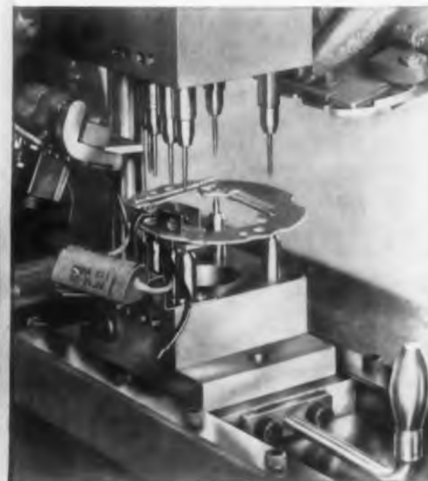
Simultaneous multiple eyeleting from either or both sides of machine. Typical six eyelet application illustrated. 50 years' experience is your assurance of complete dependability.
