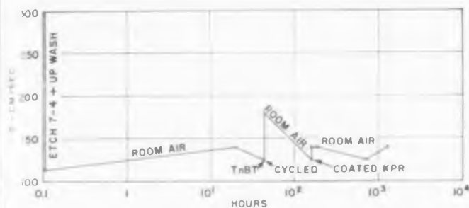
Fig. 10. Surface recombination velocity versus time in air for n-type germanium treated with tetra-n-butyl titanate and coated with a photo-resist (KPR).
