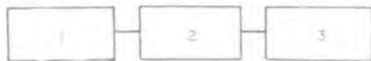
Fig. 3. Block diagram of exponential detector: 1—broadband high-pass filter; 2—nonlinear element; 3—narrow-band lowpass filter.
