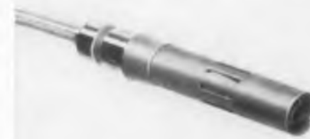
Inconel-sheathed total temperature probe mounted on Redstone missile nose cone — assures high strength at high temperatures and readily withstands oxidation, erosion and thermal shock at extreme velocities. Probe (shown at right) is product of Aero Research Instrument Company, Inc., Chicago, Illinois.
