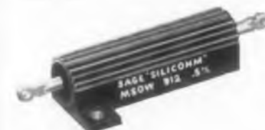
"SILICOHM" TYPE M • Metal-Clad (Chassis-Mounted) Units (10-25-50 Watts) (.1 to 175,000 ohms) to MIL-R-18546B (Ships) Specifications—Char. G.
