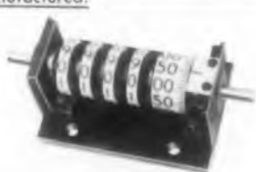
SPECIAL DECIMAL COUNTER 2660. Counts from 000000 to 999950 with return to 000000, in 50-unit increments. Input speed: 1000 rpm max. int., 300 rpm cont.; Weight: 3 oz.; Length: 2.33 in. Typical of many Bowmar designs currently being manufactured.
