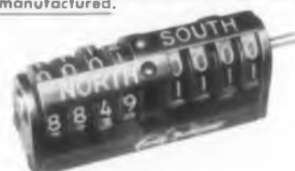
MINIATURE LATITUDE COUNTER 2417. Counts from 00°00'N to 90°00'N or S, with permissible overrun of 10°; Input speed: 1500 rpm max. int., 500 rpm cont.; Weight: 1.5 oz.; Length: 1.59 in. Typical of many Bowmar designs currently being manufactured.
