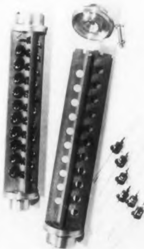
Compact rectifier package operates submerged in oil.
