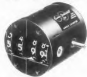
ANGLE COUNTER 1503. Counts from 000.0° to 359.9° and returns to 000.0; Input speed: 1800 rpm max. int., 500 rpm cont.; Weight: 2.5 oz.; O.D.: 1.310 in. Typical of many Bowmar designs currently being manufactured.
