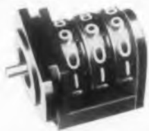
MINIATURE DECIMAL COUNTER 2416 (with servo type mounting). Counts from 000 to 999 with return to 000. Input speed: 1500 rpm max. int., 500 rpm cont.; Weight: .5 oz.; Length: .685 in. Typical of many Bowmar designs currently being manufactured.
