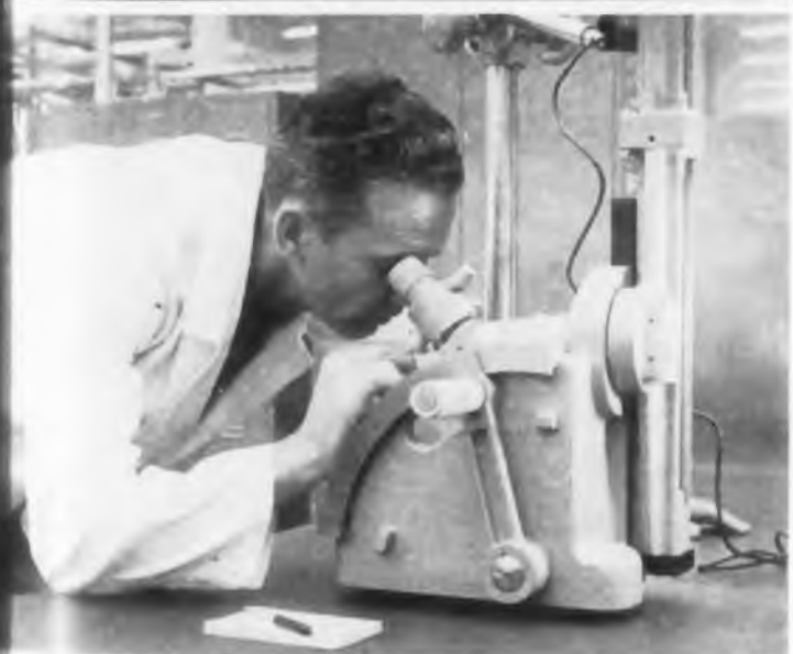
Optical gauge determines measurements within 5 millionths of an inch.
