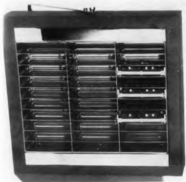
Open frame housing for modules provides efficient cooling.
