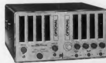
Model 202B Time-Function Translator. Frequency range, 0-220kc; input sensitivity, 0.05v rms; accuracy, \pm 1 count; time bases, 1 millisecc to 10 sec in 1 millisecc steps, 0.1 millisecc to 1 sec in 0.1 millisecc steps; price, $1100 f.o.b. factory.
