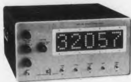
Model 211B Inline Frequency-Period Counter. Frequency range: 0-220kc; period range, 10 \mu sec to 100,000 sec; input sensitivity, 0.05v; accuracy, \pm 1 count; inline-in-plane presentation; price $1175 f.o.b. factory.
