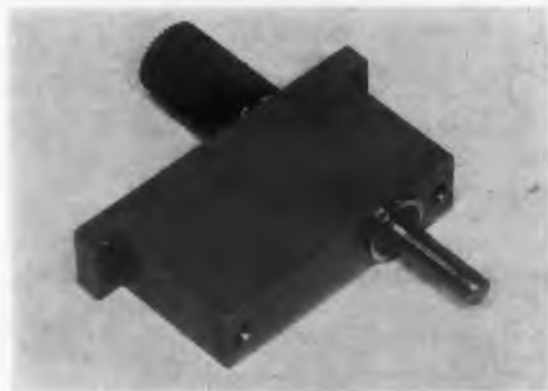
Bearing mount assembly with pinion shaft.
