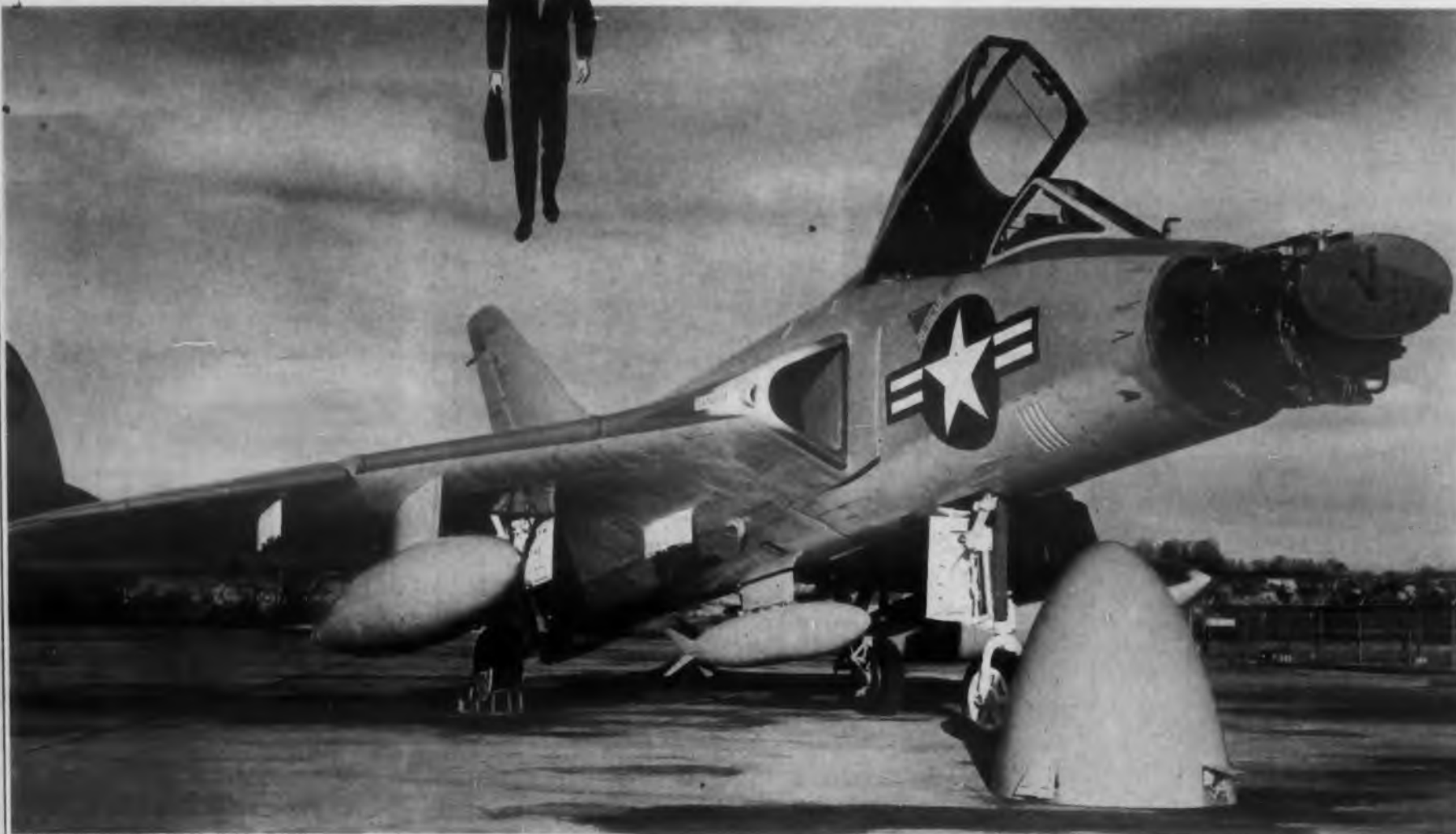
Westinghouse Aero 13 Armament Control System, mounted in nose of Navy F4D Douglas carrier-based interceptor, is typical of systems using FLEXOLON wire for faster assembly, lower production costs.
