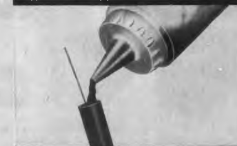
EPOXY LIQUID AND HARDENER —If application will not tolerate elevated temperatures, liquid resin and hardeners will cure at room temperature.
