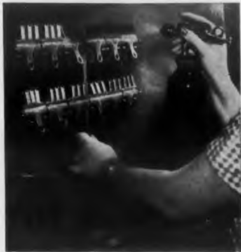
Colloidal graphite is spray-applied on grid plates to increase radiation, reduce secondary emission.
