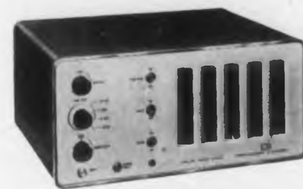
Model 201B Frequency-Period Counter. Frequency range, 0-220kc; period range, 10 \mu sec to 1 sec; input sensitivity, 0.05v; accuracy, \pm 1 count; price $700. Model 200B Frequency Counter same except no period function or crystal controlled time base; price $425 f.o.b. factory.
