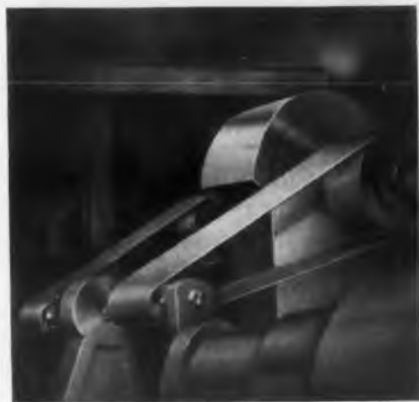
Typical application of colloidal graphite is for the elimination of static charges on drive belts.
