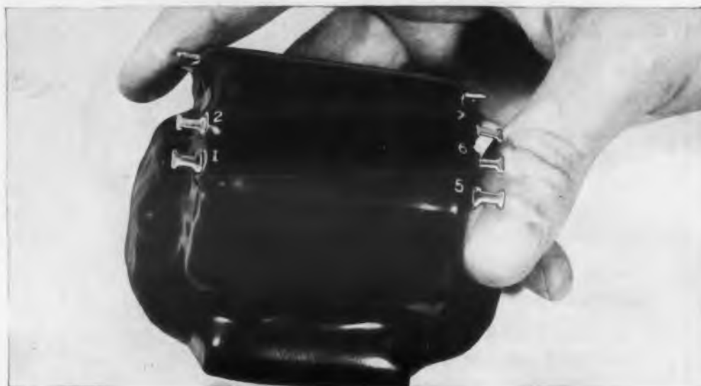
TRANSFORMER MEETING MIL-T-27A SPECIFICATIONS is shown above. This was impregnated using "SCOTCHCAST" Resin #241 and then dip-coated using new "SCOTCHCAST" Resin No. 253. There is no limit to the sizes or shapes of components that can be dip encapsulated with this heat-curing resin material.
